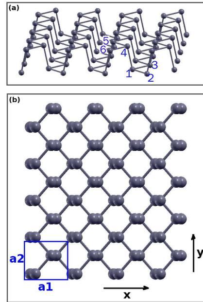
FIG. 1: (Color online) Optimized configuration of single-layer BP. Top: perspective view illustrates the pucker along the  $y$ -direction. Bottom: top view of top image showing a square lattice structure. Blue box represents the basic unit cell for single-layer BP.
