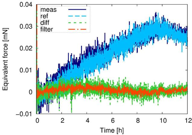
**Fig. 6** Long-term stability and resolution of the capacitive sensors: by employing both the compensation principle (difference between measuring and reference signal) as well as the mathematical filtering of oscillations (smoothing) the theoretically constant signal stays within a measuring corridor of  $10\ \mu\text{N}$  (converted from voltage). This value coincides the required resolution based on theoretical considerations (see text).
