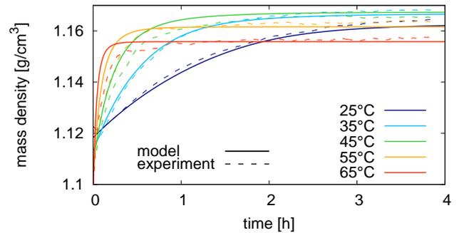
**Fig. 8** Volumetric changes due to curing: comparison of experimental data (dashed) and simulation data for different time-temperature regimes. Both graphs are obtained after numerical treatment of Eq. (13) and (15).
