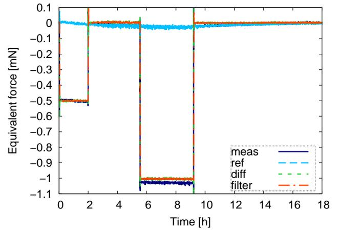
**Fig. 7** Long-term behaviour of the test rig with temporary applied constant loads: the setup shows linear behaviour, the compensation of environmental influences (like temperature changes and air flow) works properly and the mathematical filter (smoothing) reduces the overshooting effects.
