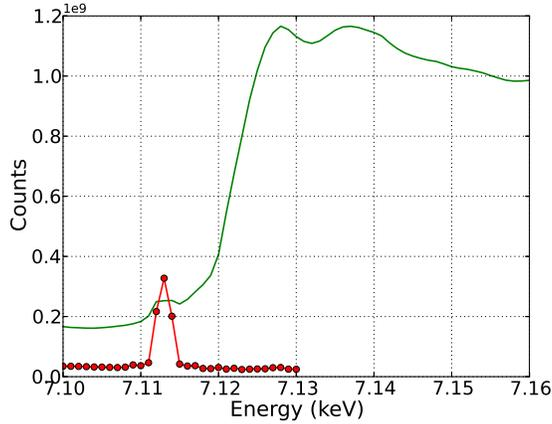
FIG. 6. The absorption (fluorescence) spectrum of  $\text{FeBO}_3$  near the Fe  $K$  edge (green line), showing a weak pre-edge peak. Red: the resonant (003) forbidden scattering spectrum, showing a single sharp peak at the absorption pre-edge position.
