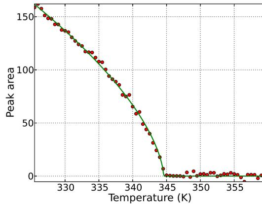
FIG. 5. The (003) magnetic diffraction intensity at 5.1 keV with a field angle of  $90^\circ$  vs temperature, across the magnetic phase transition. The solid line is a power-law fit to the function  $I \propto |M|^2 \propto (T_N - T)^{2\beta}$ , giving  $\beta = 0.305(2)$ .
