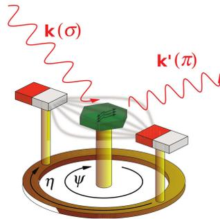
FIG. 2. A schematic of the experiment, showing the incident and scattered x-ray beams and the  $\text{FeBO}_3$  crystal with weak ferromagnetic moments directed along the direction of the applied magnetic field. Sample and field were rotated about a common axis so that  $\psi = 0$  and  $\eta = 0$  correspond to the the crystallographic  $(100)_{hex}$  axis, and field direction (from south to north pole of the magnet assembly), directed along  $\mathbf{k} + \mathbf{k}'$ , respectively.
