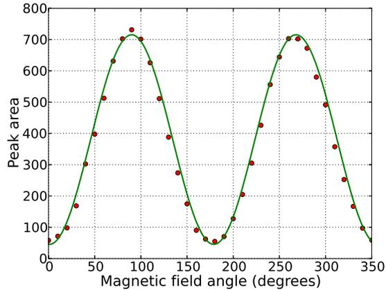
FIG. 4. The dependence of the non-resonant magnetic (003) Bragg reflection intensity on the magnetic field angle ( $B \simeq 0.011$  T), measured at an energy of 5.1 keV. Red circles are data points and the calculated spin-scattering intensity is shown by a solid green line.
