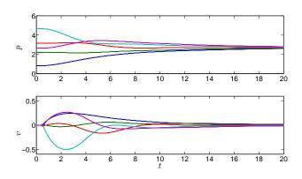
Fig. 2. Evolution of  $p_i$  (top) and  $v_i$  (bottom) for b = 10 using the event-triggered controllers,  $i \in \{1, ..., N\}$ .
