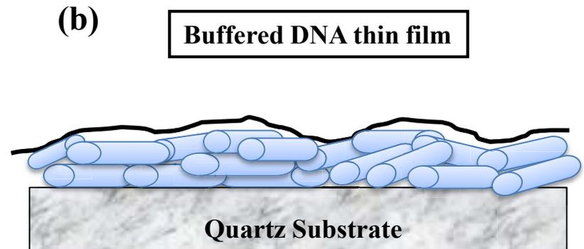
**Figure 3:** Schematic structure of pristine (a) and buffered (b) film based on our model.
