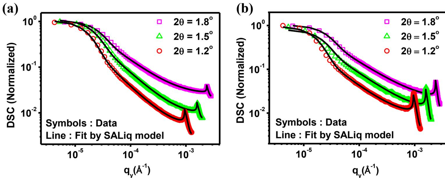
**Figure 2:** Transverse diffuse scattering data taken at different detector angles ( $2\theta$ ): (a) pristine film and (b) buffered DNA film. DSC stands for Differential Scattering Cross-section. The symbols denote data points whereas lines denote fit by self-affine liquid model under DWBA scheme.
