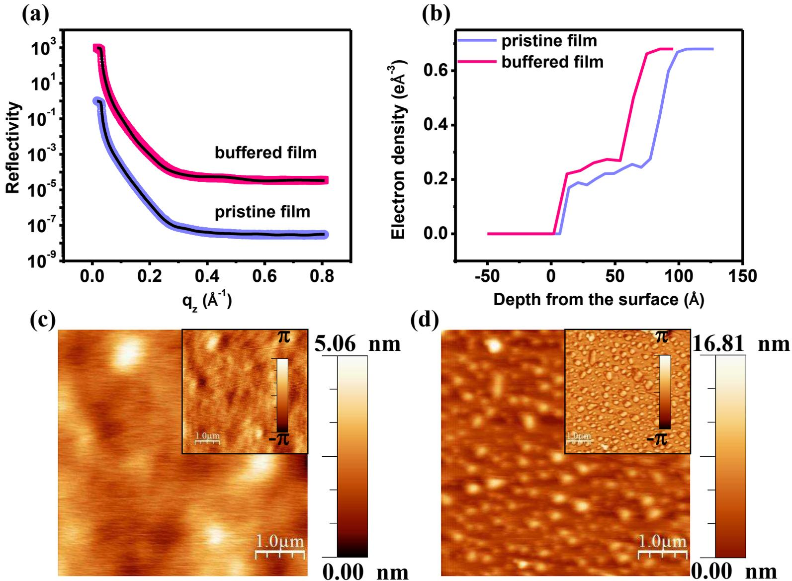
**Figure 1:** Pristine and buffered DNA films: (a) X-ray reflectivity profiles of pristine and buffered DNA films, fit with DWBA formalism (up shifted for clarity). Symbols: experimental data points; line: fit, (b) Corresponding EDPs, (c) AFM image of pristine film (scan size  $5\mu\text{m} \times 5\mu\text{m}$ ), (d) AFM image of buffered film (scan size  $5\mu\text{m} \times 5\mu\text{m}$ ). Insets of (c) and (d) show corresponding phase images.
