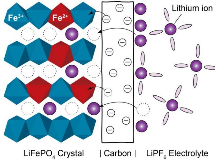
**Figure 1. Schematic demonstration of the interface of a carbon-coated  $\text{Li}_x\text{FePO}_4$  crystal.** Lithium ions in the electrolyte jump across the carbon coating into the vacancies in the first atomic layer of the crystal, while electrons in the carbon coating tunnel to the adjacent iron site to reduce the  $\text{Fe}^{3+}$  ions. ( $\text{PO}_4$  tetrahedrons are omitted for clarity.)
