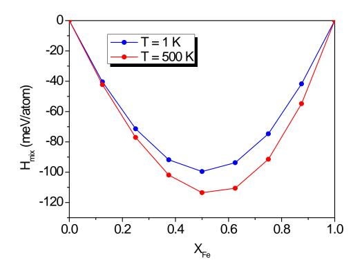
Figure 5. Enthalpy of mixing of random fcc Fe-Ni alloy configurations computed for low and high temperatures T=1 K and T=500 K.
