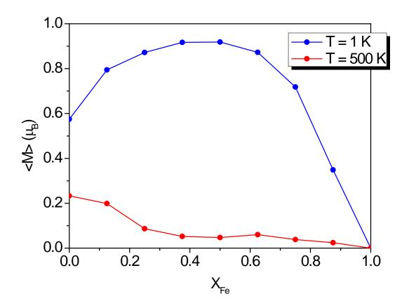
Figure 7. The total magnetic moment of a random Fe-Ni mixture plotted as a function of Fe content at a very low temperature and at T = 500 K.
