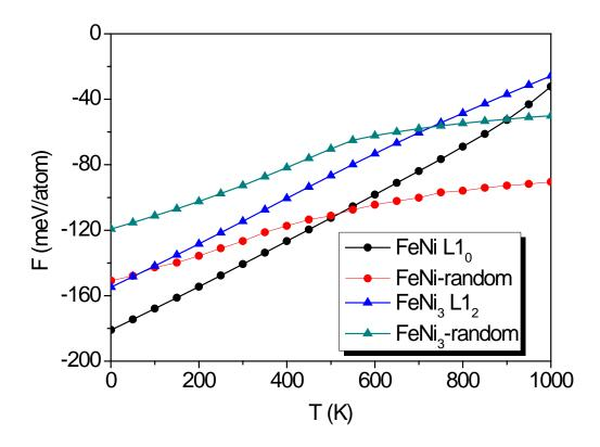
Figure 11. Comparison of free energies of ordered and random structures simulated using MCE for stoichiometric compositions FeNi and FeNi<sub>3</sub>.
