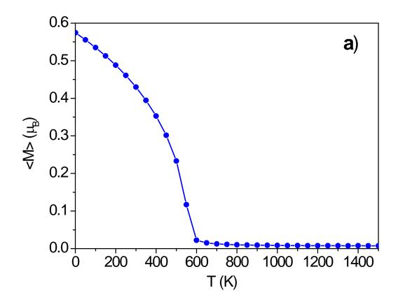
Figure 4a. Magnetic moment of pure nickel  $(\mu_B)$  plotted as a function of temperature.
