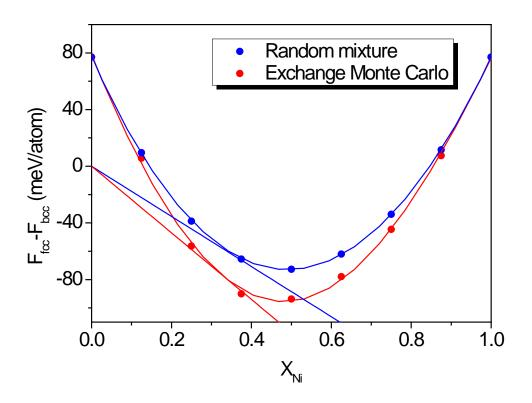
Figure 9. Tangent construction defining the coexistence curve between bcc Fe and fcc Fe-Ni alloys at temperature T=600 K.
