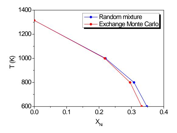
Figure 10. Coexistence curves between bcc Fe and fcc Fe-Ni alloys. The blue line corresponds to random alloys, the red line was computed using exchange Monte Carlo simulations.
