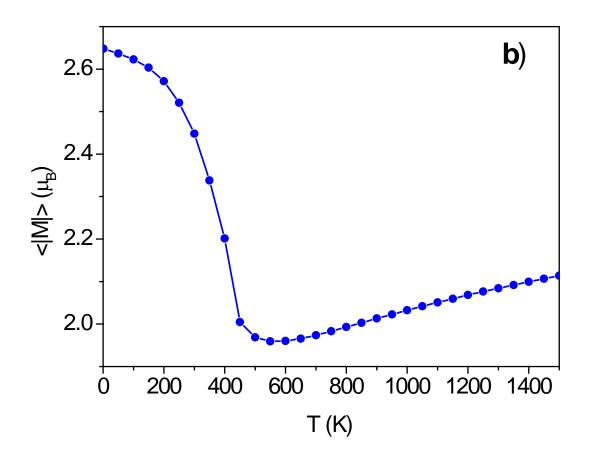
Figure 3b. Average length of atomic magnetic moment in fcc Fe  $(\mu_B)$  plotted as a function of temperature.
