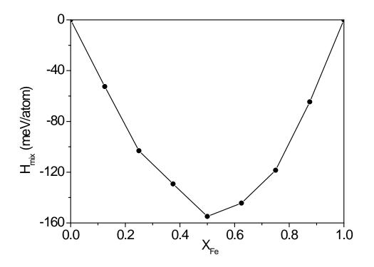
Figure 6. Enthalpy of mixing of FeNi alloys plotted as a function of Fe content for quenched configurations.
