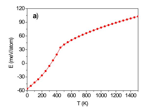
Figure 3a. Energy of pure fcc iron (in meV/atom units) plotted as a function of temperature.
