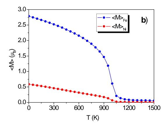
Figure 8b. Magnetic moments of Fe and Ni sublattices in an ordered FeNi alloy plotted as a function of temperature.
