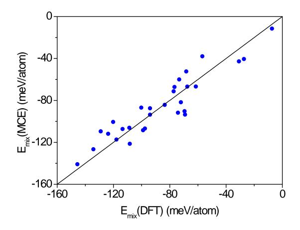
Figure 2. Comparison of DFT and MCE energies of mixing for the alloy configurations used for fitting the MCE Hamultonian.
