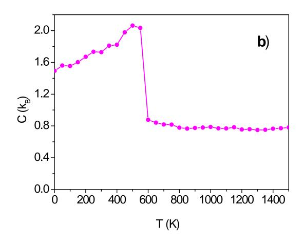
Figure 4b. Temperature dependence of the magnetic part of the specific heat computed using MCE for pure nickel.
