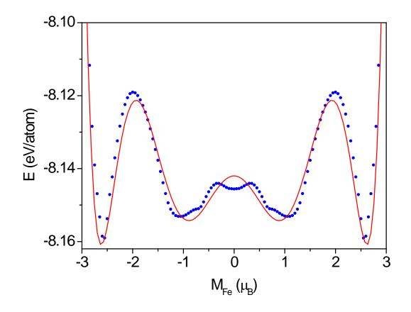
Figure 1. Comparison of DFT (points) energies of ferromagnetic fcc Fe plotted as a function of magnetic moment, and the MCE Landau expansion (line), which includes terms up to the 8<sup>th</sup> order in atomic magnetic moment.
