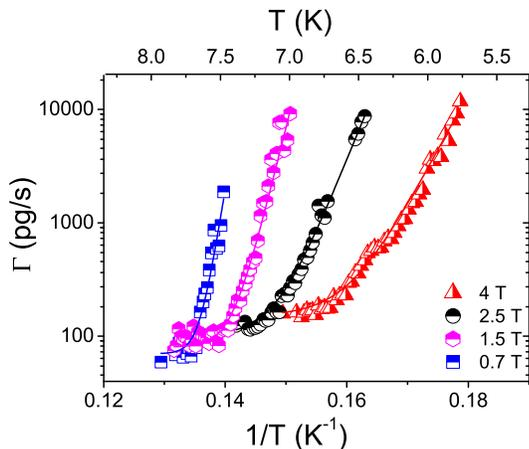
FIG. 2. Temperature evolution of the cantilever energy dissipation, measured after field-cooling, at different fields. The upturn of  $\Gamma$  marks the onset of the superconductivity transition, as discussed in the text. The solid lines are the best fits to equation 7.
