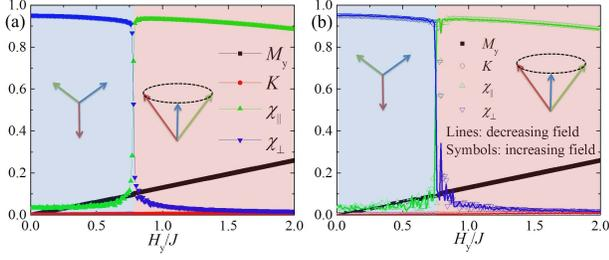
FIG. 2. (color online) (a) Different observables as a function of  $\mathbf{H} \parallel \hat{y}$  obtained from equilibrium simulations. (b) Similar to (a) but obtained by sweeping the magnetic field. Here  $T = 0.02J$  and  $M_y$  is the total magnetization along the field direction.
