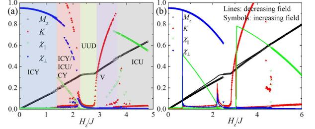
FIG. 3. (color online) (a) Magnetic field dependence of different observables for  $\mathbf{H} \parallel \hat{z}$  in equilibrium simulation. Due to the nature of the first order phase transition, several phases can coexist in certain magnetic field region. (b) Same as (a) but obtained with sweep of magnetic fields. Here  $T = 0.02J$  and  $M_z$  is the total magnetization along the field direction.
