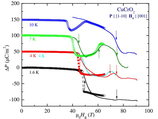
FIG. 5. (color online)  $\mathbf{P}$  vs  $\mathbf{H}_a$  data measured on the upsweep of a 65 T capacitor-driven magnet (points) [18] and with shots up to 92 T in the 100 T multi-shot magnet (lines, this work). The variation with  $H_a$  sweep rate is discussed in the text and the Supplemental Information. [25] Arrows indicate phase transitions based on the 92 T data shown as blue points in Fig. 4
