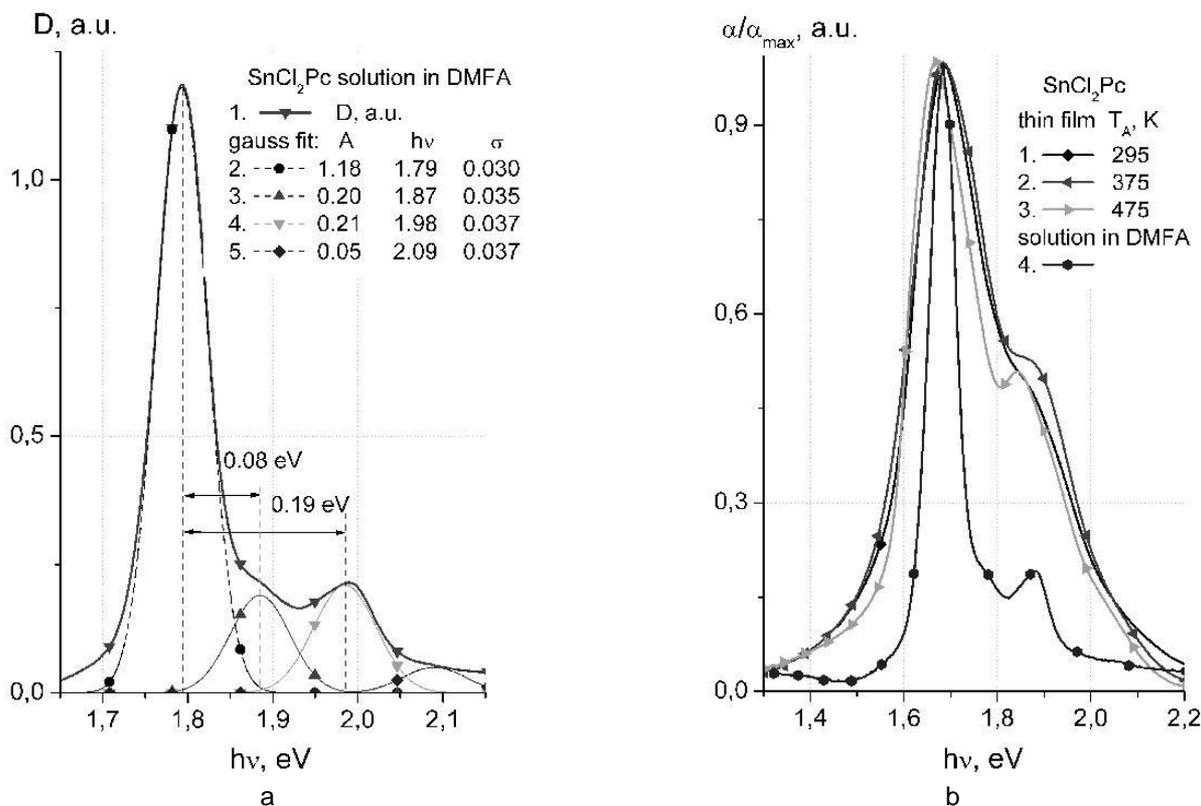
Fig. 1. *a* Spectral dependence of the optical density,  $D$ , of an  $\text{SnCl}_2\text{Pc}$  solution in DMFA (1) and the Gauss fit (2-5); *b* AS normalized on the maximum of  $\text{SnCl}_2\text{Pc}$  films with thickness 180 nm before (1) and after annealing at  $T_a = 375$  K (2), 475 K (3) and the  $\text{SnCl}_2\text{Pc}$  solution in DMFA (4) is red-shifted by 0.12 eV
