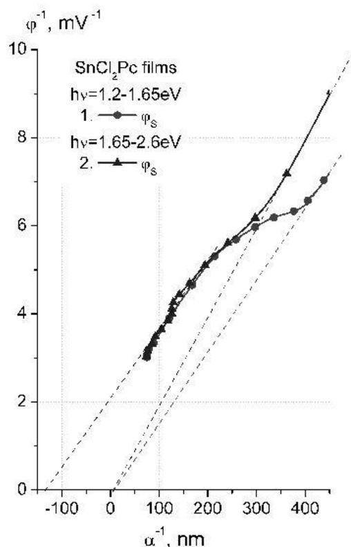
Fig. 6. Dependence of  $\varphi^{-1}(\alpha^{-1})$  in the ranges 1.20-1.65 eV (1) and 1.65-2.60 eV (2) at the illumination of the free surface of ITO/SnCl<sub>2</sub>Pc structures
