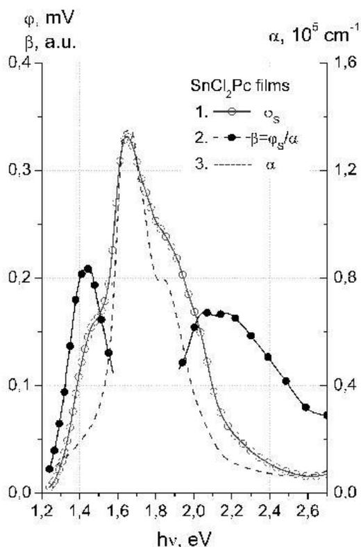
Fig. 5. Spectral dependence of photovoltage,  $\varphi$ , (1) absorption coefficient,  $\alpha$ , (2), and quantum efficiency,  $\beta$ , (3) of ITO/SnCl<sub>2</sub>Pc structures
