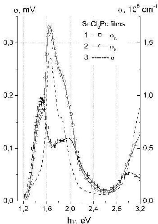
Fig. 3. Spectral dependence of photovoltage at illumination of ITO contact,  $\varphi_c$ , (1) and free surface,  $\varphi_s$ , (2) and absorption coefficient,  $\alpha$ , (3) of ITO/SnCl<sub>2</sub>Pc structures at  $T_s = 415$  K
