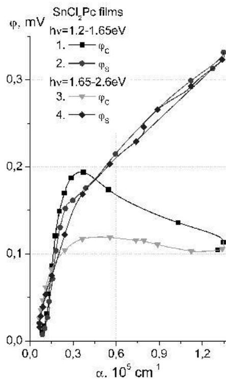
Fig. 4. Dependence of the photovoltage on the absorption coefficient,  $\varphi(\alpha)$  at the illumination of the ITO contact (1,3) and the free surface (2,4) of ITO/SnCl<sub>2</sub>Pc structures in the ranges 1.20-1.65 eV (1,2) and 1.65-2.60 eV (3,4)
