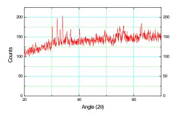
Fig.5: X-ray pattern of Zn-Sn substituted barium hexaferrite after heat treatment.
