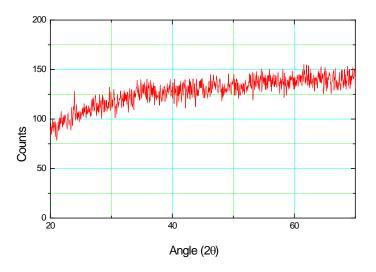
Fig.1: X-ray pattern of barium hexagonal ferrite before heat treatment.
