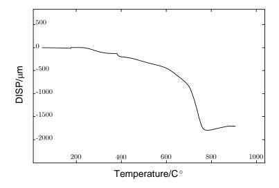
Fig.3: A dilatometer curve of a pellet of the green body.
