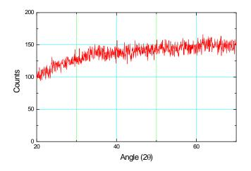
Fig.4: X-ray pattern of Zn-Sn substituted barium hexaferrite before heat treatment.
