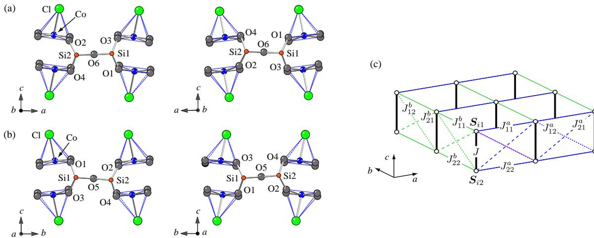
**Fig. S8.** Atomic configuration between neighboring dimers (a) along the  $a$  direction and (b) along the  $b$  direction. (c) A model of exchange network for  $\text{Ba}_2\text{CoSi}_2\text{O}_6\text{Cl}_2$ . Thick solid lines represent the intradimer exchange interaction  $J$ , and thin solid, dashed and dotted lines represent the interdimer exchange interactions  $J_{\alpha\beta}^a$  and  $J_{\alpha\beta}^b$  ( $\alpha, \beta = 1, 2$ ).
