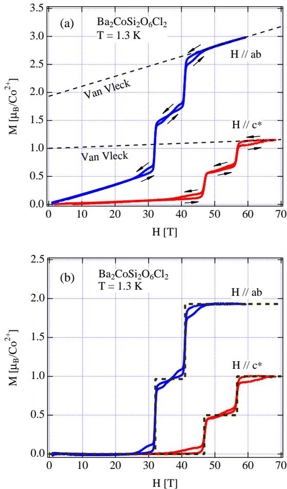
**Fig. 3.** (Color online) (a) Raw magnetization curves measured at 1.3 K for  $H \parallel c^*$  and  $H \parallel ab$  using a piece of single crystal. Arrows indicate the route of the magnetization process upon sweeping the field up and down. (b) Magnetization curves corrected for Van Vleck paramagnetism. Dashed lines are theoretical magnetization curves calculated using eq. (2) with the parameters given in the text.
