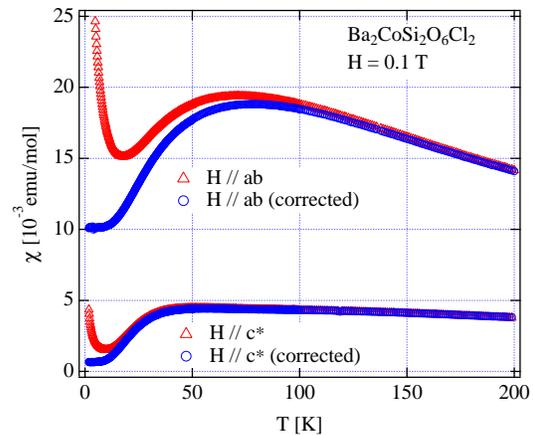
**Fig. 2.** (Color online) Magnetic susceptibilities in  $\text{Ba}_2\text{CoSi}_2\text{O}_6\text{Cl}_2$  measured at  $H = 0.1$  T for  $H \parallel c^*$  and  $H \parallel ab$ . Red and blue symbols are raw data and the data corrected for the Curie term.
