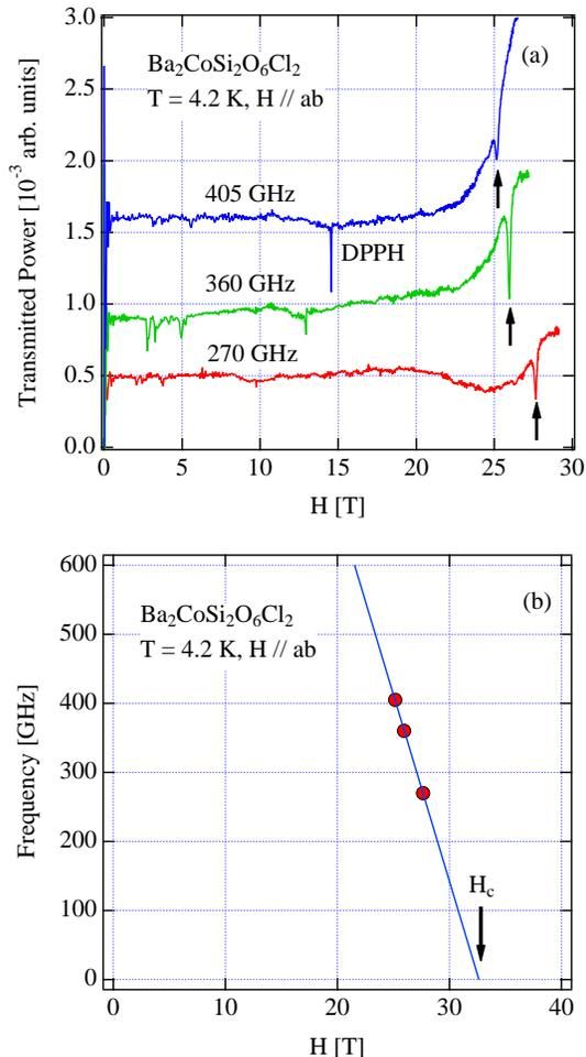
**Fig. 4.** (Color online) (a) ESR absorption spectra in  $\text{Ba}_2\text{CoSi}_2\text{O}_6\text{Cl}_2$  measured at  $T = 4.2$  K for  $H \parallel ab$ . Arrows are resonance fields for singlet-triplet transitions. (b) Frequency vs field diagram of ESR mode measured for  $H \parallel ab$ . The solid line is a linear fit for the singlet-triplet transitions with  $g_{ab} = 3.86$ .
