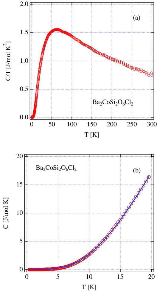
**Fig. 5.** (Color online) (a) Specific heat divided by the temperature measured at zero magnetic field. (b) Low-temperature specific heat. The solid line is a fit based on the isolated dimer model with  $J^\perp/k_B = 105$  K and  $J^\parallel/J^\perp = 0.149$  (fixed).
