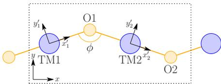
FIG. 1: (Color online) Schematic diagram of corner-sharing TM-O system, which for bond-angle  $\phi$  not equal to  $180^\circ$  lacks inversion symmetry at the oxygen site. The  $z$ -direction is out of plane.
