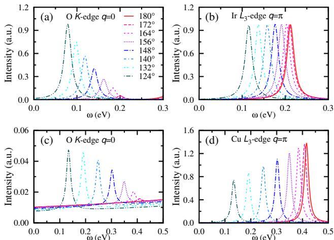
FIG. 2: (Color online) Magnetic RIXS spectra calculated by ED as a function of TM-O-TM bond angle  $\phi$ . (a) Iridate O  $K$ -edge at  $q = 0$ , (b) Ir  $L_3$ -edge at  $q = \pi$ , (c) Cuprate O  $K$ -edge RIXS at  $q = 0$ , (d) Cu  $L_3$ -edge at  $q = \pi$ . The polarizations are  $\epsilon = x$  and  $\epsilon' = z$ . Note that as a function of  $\phi$  both the effective magnetic interactions and the RIXS intensity change.
