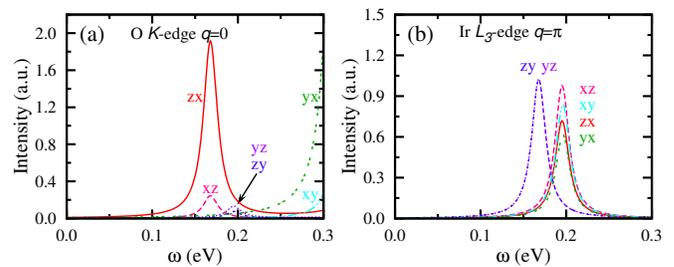
FIG. 3: (Color online) Polarization dependence of magnetic RIXS excitations for an iridate cluster with an Ir-O-Ir bond-angle of  $\phi = 158^\circ$ . (a) O  $K$ -edge at  $q = 0$ , (b) Ir  $L_3$ -edge at  $q = \pi$ . The polarization condition  $zx$  labels  $\epsilon = z$ ,  $\epsilon' = x$ .
