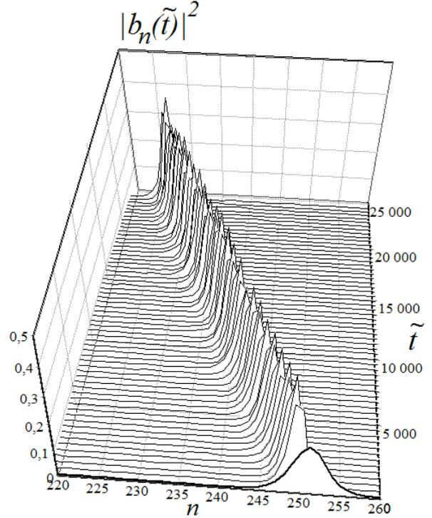
Figure 3: Graphs of the function  $|b_n(\tilde{t})|^2$  for the above-cited values of the chain parameters at  $\xi = 2.2$  and the electric field intensity  $\mathcal{E} = 7.52 \cdot 10^4 \text{V/cm}$ ,  $\tilde{t} = 0 \rightarrow 25000$ . The chain length is  $N = 1700$  sites.
