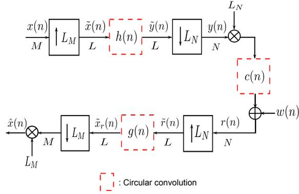
Fig. 10: SC-FDMA equivalent time domain system model
