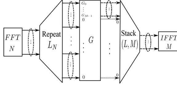
Fig. 7: Localised demapping and equalization equivalent model
