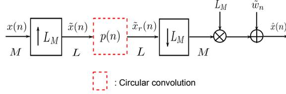
Fig. 18: SC-FDMA simplified system model
