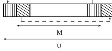
Fig. 12: Copying from a length  $M$  to  $U \leq 2M$
