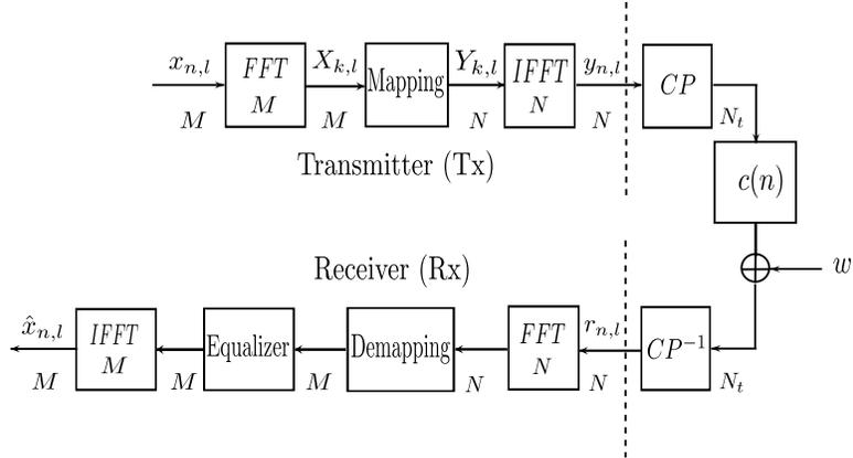
Fig. 1: SC-FDMA frequency based scheme representation
