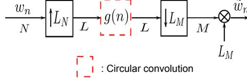
Fig. 19: Equivalent noise
