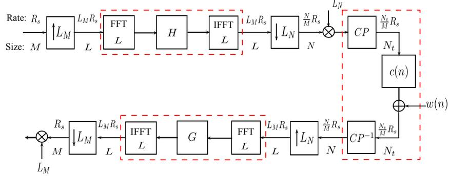
Fig. 9: SC-FDMA equivalent frequency domain system model
