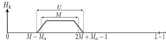
Fig. 14: Spectral shaping filter with root raised cosine
