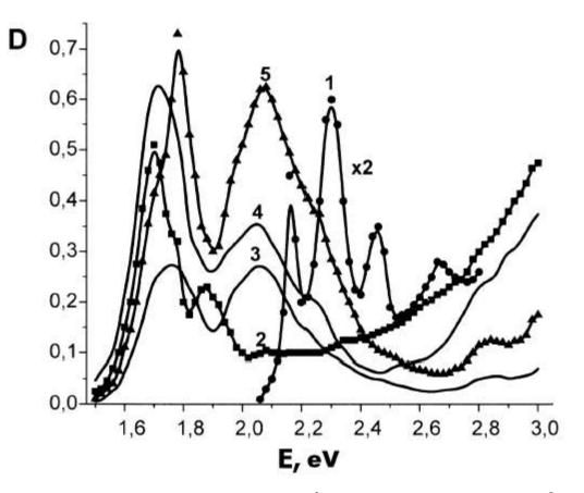
Fig. 2. Absorption spectra of Pn (curve 1, C =  $4.0 \times 10^{-6}$  mol/l) and HTPn (curve 2, C =  $1.0 \times 10^{-5}$  mol/l) solutions in trichlorobenzene; and of PTPn in benzene (curve 3, C =  $5.4 \times 10^{-6}$  mol/l), trichlorobenzene (curve 4, C =  $1.2 \times 10^{-5}$  mol/l), and DMFA (curve 5, C =  $1.4 \times 10^{-5}$  mol/l)
