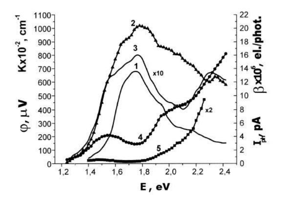
Fig. 5. Various spectra of PTPn films, 560 nm in thickness each: absorption (1); CPV ( $\phi$ ) under frontal (2) and back (3) modulated illumination; photocurrent lph (4) and quantum efficiency  $\beta$  (5) under fixed illumination
