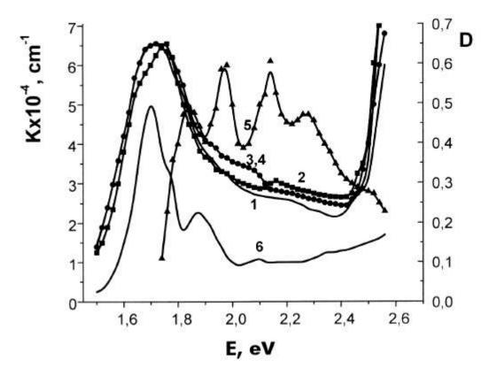
Fig. 3. Absorption spectra of HTPn (PTPn1) 100-nm films on quartz substrates (curves 1 to 4), a Pn 400-nm film (curve 5) [17], and a HTPn solution in trichlorobenzene (curve 6)
