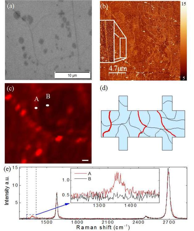
FIG. 5. (a) Optical and (b) atomic force microscopies. (c) Raman D peak map (scale bar is 1.5  $\mu m$ ). Figures (a)-(c) concern about the same area of sample S2. (d) Representation of the network of line defects corresponding to short-circuit paths between the sample edges. (e) Raman signal on (A) and away (B) from a wrinkle. Inset: zoom in the D peak zone of the Raman spectra.
