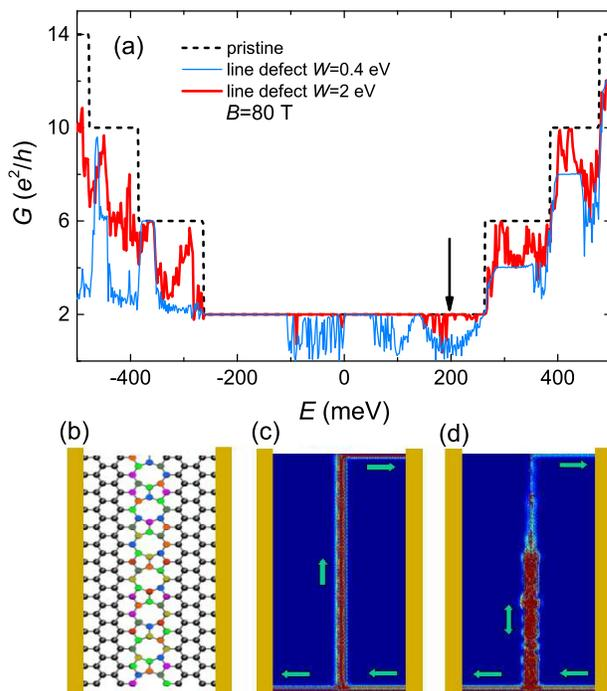
FIG. 6. (a) Two-terminal magnetoconductance of a pristine aGR, and of aGR with a 8-5 line defect crossing the sample (represented in (b)) including a random disorder potential of  $W = 0.4$  eV (blue line) and  $W = 2$  eV (red line). (b) Representation of the 8-5 line defect crossing the aGR. (c) and (d) spatial distribution of the electrons injected from the source contact (to the right) at 200 meV is shown in insets (c)  $W = 0.4$  eV and (d)  $W = 2$  eV.
