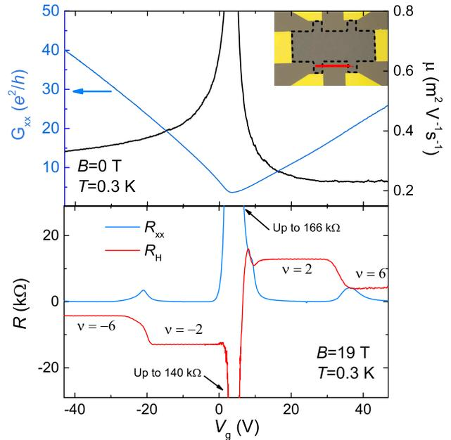
FIG. 1. (a) Longitudinal conductance and carrier mobility vs.  $V_g$  and (b)  $R_H$  and  $R_{xx}$  vs.  $V_g$  for sample S1. Insert in (a): Hall bar optical image. The length scale (red segment) between voltage terminals is  $200 \mu\text{m}$  and equal to the Hall bar width.
