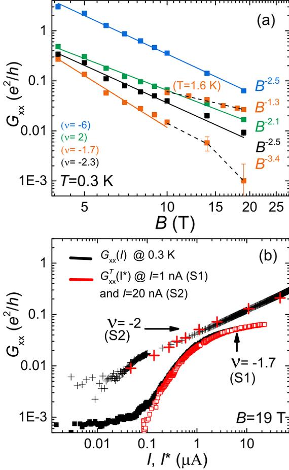
FIG. 4. (a)  $G_{xx}$  vs.  $B$  in log-log scale at 0.3 K for different filling factors for S1. (b)  $G_{xx}$  vs.  $I$  and  $G_{xx}^T$  vs.  $I^*$  in log-log scale for the two samples with  $I^*[A] = 0.87 \times 10^{-6} T[K]^{1.74}$  for S1 and  $I^*[A] = 0.6 \times 10^{-6} T[K]^{2.1}$  for S2.
