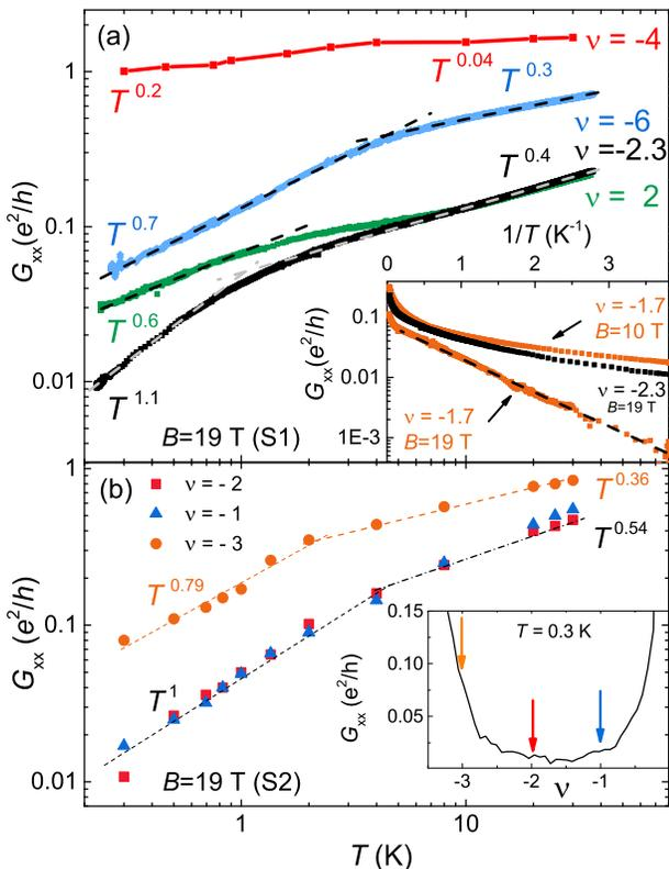
FIG. 3. (a)  $G_{xx}$  vs.  $T$  in log-log scale at 19 T for S1. Inset:  $G_{xx}$  in log scale vs.  $1/T$  for  $\nu = -1.7$  at 19 and 10 T and at  $\nu = -2.3$  for comparison. (b)  $G_{xx}$  vs.  $T$  in log-log scale for S2. Inset:  $G_{xx}$  vs.  $\nu$  at 0.3 K, arrows indicate the values of  $\nu$  at which measurements are performed.
