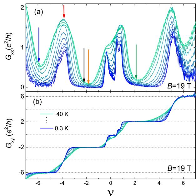
FIG. 2. (a)  $G_{xx}$  and (b)  $G_{xy}$  vs.  $\nu$  for  $T$  between 0.3 K and 40 K at 19 T, obtained in sample S1. Temperature color code apply for both figures. Arrows in (a) indicate the values of  $\nu$  at which measurements in Fig. 3(a) are performed.
