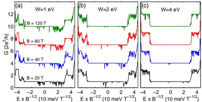
FIG. 9. Two-terminal magnetoconductance of a 200 nm wide graphene ribbon with a disordered 5-8 line defect under different magnetic fields. The strength of the disorder  $W$  is 1 eV (a), 2 eV (b), 4 eV (c). The base lines were shifted for the sake of clarity.
