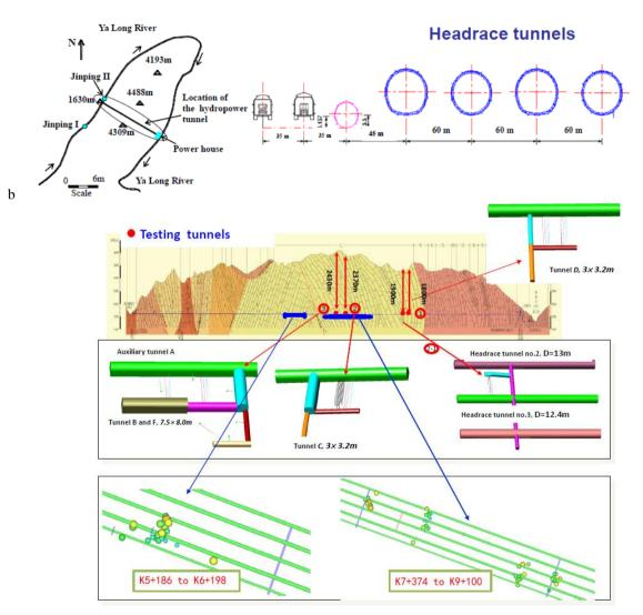
Fig. 2. Schematics of JinPing tunnel complex: (a) location and cross-sections of seven tunnels ; (b) additional small test tunnels located in the central portion of large diameter main tunnels (12.4 -13 m for the two headrace tunnels shown) and examples of micro-seismic events measured along the tunnels, from Feng (2011), slides 9 and 11.
