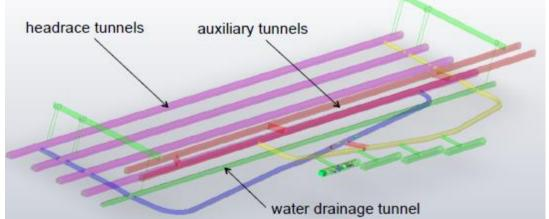
Fig. 3. Schematic diagram of CJPL-II: (a) Eight lab spaces connected by four 60 m long access drifts; (b) 3-D prospective of CJPL-II in relation to the JinPing tunnel complex, from Li (2013a) slides 79-80 or Li (2013b) slide 25.
