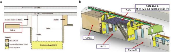
Fig. 1. Schematic diagram displaying features of CJPL-I: (a) Floor plan of Halls A (physics experiments) and B (rock mechanics studies), and an early proposal for future expansion (C); (b) Layout of the CDEX and Panda-X in Hall A and associated supporting equipment, from Yue and Wong (2013), Fig. 1, and Li (2013a), slide 55.
