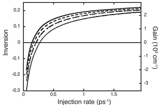
FIG. 11. Population inversion and gain for the QD transitions versus injection rate for structure B. The carrier density referring the pump distribution is  $N^F = 6 \times 10^{10} \text{ cm}^{-2}$  (solid line),  $N^F = 5 \times 10^{10} \text{ cm}^{-2}$  (dashes line),  $N^F = 4 \times 10^{10} \text{ cm}^{-2}$  (dot-dashed line) and  $N^F = 3 \times 10^{10} \text{ cm}^{-2}$  (dotted line). The lattice temperature is 150 K.
