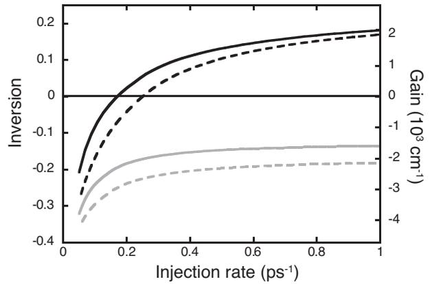
FIG. 8. Population inversion and gain for the QD transitions versus injection rate for structure A (gray lines) and structure B (black lines). The lattice temperature is 150 K (solid line) and 300 K (dashed line).
