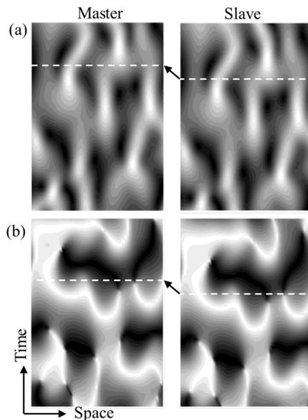
FIG. 2: Spatiotemporal dynamics of (a) amplitude and (b) phase of the master and the slave systems for two unidimensional complex Ginzburg-Landau systems coupled as in Eqs.(5-6). Parameter values:  $\tau = 0.6$ ,  $\theta = \frac{\pi}{4}$ ,  $K = 0.6$ ,  $N = 64$ ,  $\delta x = 0.2$ ,  $\delta t = 2 \times 10^{-3}$ ,  $c_1 = 3$ ,  $c_2 = -2.5$  (in a range of defect turbulence regime). The difference in time between the horizontal dashed lines is the anticipation time  $\tau = 0.6$ .
