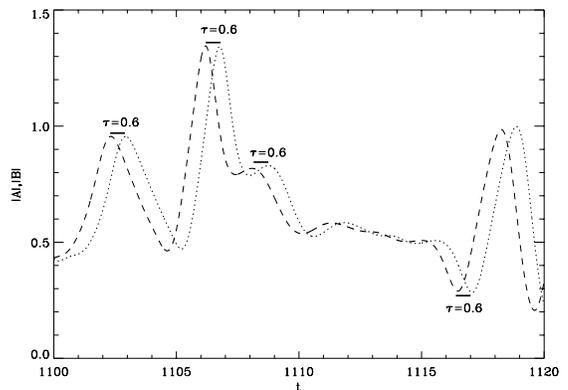
FIG. 3: Time series of the master amplitude  $|A|$  (dotted line) and the slave  $|B|$  (dashed line) for the complex Ginzburg-Landau equation in the defect turbulence regime. Horizontal arrows mark the anticipation time. Same parameters as in Fig.2.
