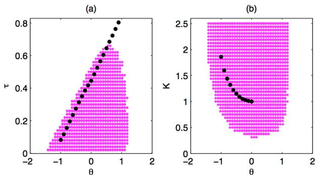
FIG. 5: (color online) Purple dots indicate the projections in the planes (a)  $(\tau, \theta)$  and (b)  $(K, \theta)$  of the region for which stable anticipated synchronization solutions have been found numerically in the defect turbulence regime with parameters  $(c_1, c_2) = (3, -2.5)$ . The black-dotted lines are the analytical results obtained from an approximate linear stability analysis, see Eq.(17).
