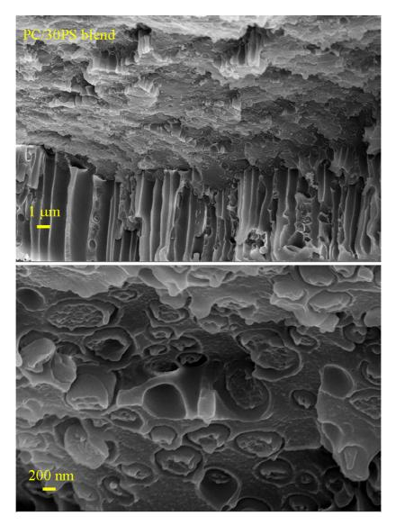
Figure 2 SEM images of cryo-fractured surface of pristine PC/30PS blend at different magnifications.
