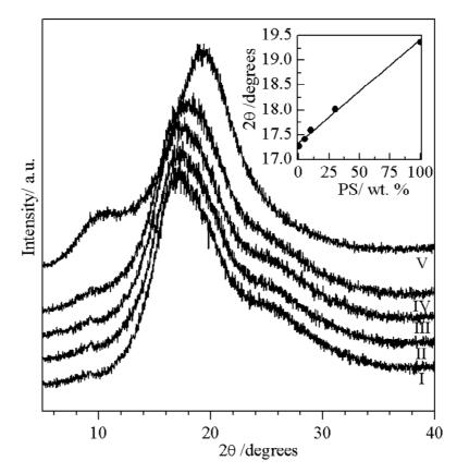
Figure 4 XRD pattern of: (I) pure PC, (II) PC/5PS, (III) PC/10PS, (IV) PC/30PS blends, and (V) pure PS. Inset shows peak position of characteristic PC peak as a function of PS content.
