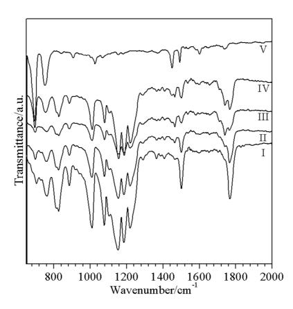
Figure 3 FTIR spectra of: (I) pure PC, (II) PC/5PS, (III) PC/10PS, (IV) PC/30PS blends, and (V) pure PS.
