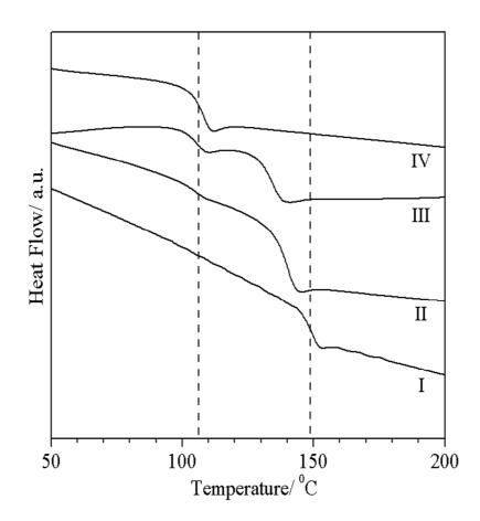
**Figure 5** DSC thermograms of: (I) pure PC, (II) PC/10PS + 3%C15A and (III) PC/30PS + 3%C15A blends, and (IV) PS.
