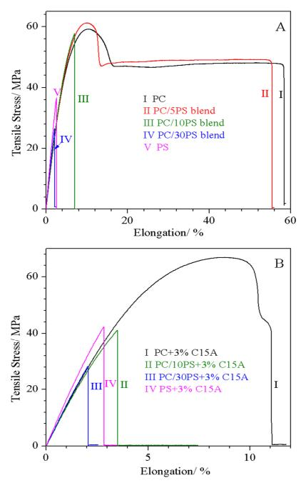
Figure 9 Stress-strain behavior of (A) Pristine PC/PS blends, (B) PC/PS +3% C15A organoclay.
