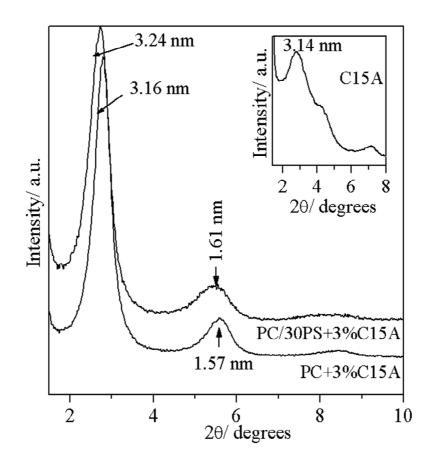
**Figure 7** XRD patterns of PC + 3%C15A and PC/30PS + 3%C15A nanocomposite. Inset shows XRD pattern of pure C15A organoclay.
