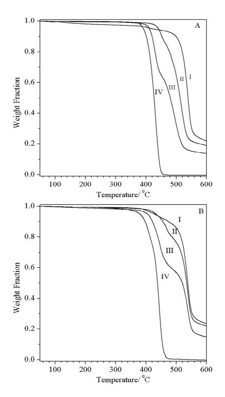
**Figure 8** TGA thermograms of: (I) pure PC, (II) PC/10PS, (IV) PC/30PS blends, and (V) PS (A) without and (B) with 3%C15A organoclay.
