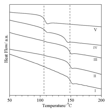
**Figure 1** Second run DSC thermograms of: (I) pure PC, (II) PC/5PS, (III) PC/10PS, (IV) PC/30PS blends, and (V) pure PS.
