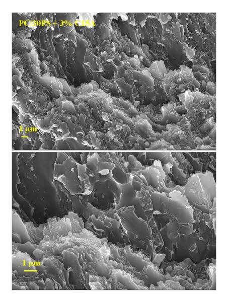
**Figure 6** SEM images of cryo-fractured surface of PC/30PS+3%C15 blend at different magnifications.
