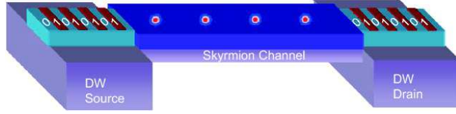
FIG. 5. A hybrid device based on DWs and skyrmions. A sequence of information ( i.e. , data bits) is encoded as a train of DWs and then converted into a train of skyrmions, which is transmitted in the skyrmion channel. We read out the information by converting skyrmions back to DWs.
