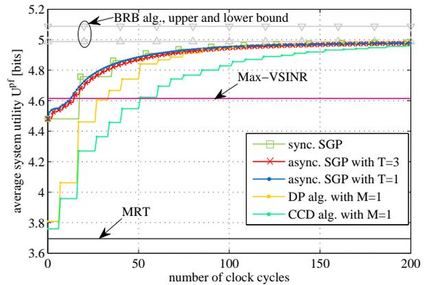
Fig. 7. Comparison of synchronous and asynchronous algorithms for NW3 with  $D = 3$ . The plot shows the system utility  $U^{Pf}$  as a function of the time index. The results are averaged over 100 channel realizations.
