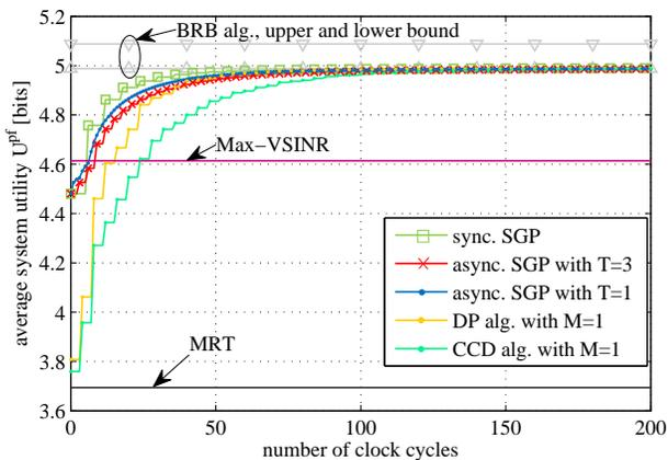
Fig. 5. Comparison of synchronous and asynchronous algorithms for NW1 with  $D = 3$ . The plot shows the system utility  $U^{Pf}$  as a function of the time index. The results are averaged over 100 channel realizations.
