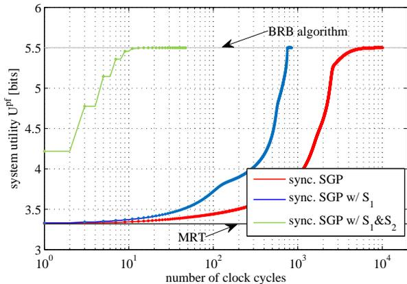
Fig. 4. Comparison of different speed-up methods for the sync. SGP. The plot shows the system utility  $U^{Pf}$  as a function of the time index for a mesh backhaul network with communication delay  $D = 1$ .
