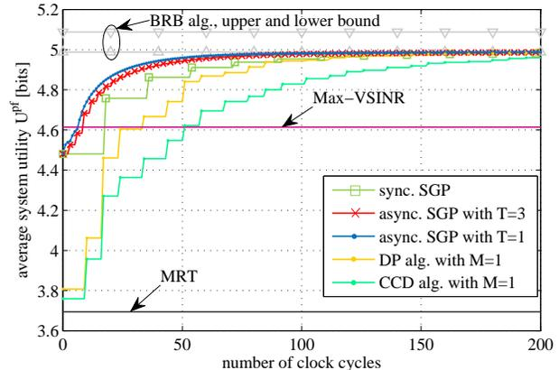
Fig. 6. Comparison of synchronous and asynchronous algorithms for NW2 with  $D = 3$ . The plot shows the system utility  $U^{Pf}$  as a function of the time index. The results are averaged over 100 channel realizations.
