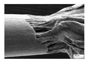
Fig. 24. Niobium filaments after etching of copper matrix of *CuNb15k* composite of diameter 0.15 mm
