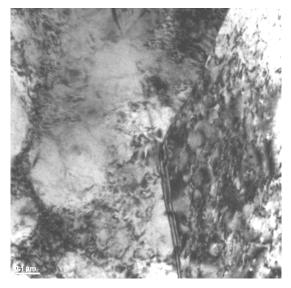
Fig. 5. Microstructure of the deformed wire from *CuAg15* alloy TEM, longitudinal section.
