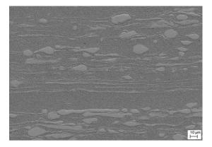
Fig. 13. Microstructure of CuNb15 alloy wire after drawing to diameter of 0.5 mm and after annealing in temperature of 700 °C for 3 hours, section parallel to drawing direction.
