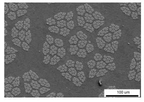
Fig. 19. Part of a section of *CuNb15k* after seventh compacting stage, wire diameter 0.15 mm.
