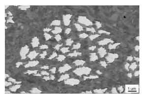
Fig. 20. Microstructure of *CuNb15k* composite. Conspicuous sections of niobium filaments in microcrystalline copper matrix.
