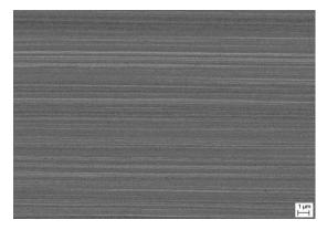
Fig. 4. Microstructure of *CuAg15* alloy wire (longitudinal section) of diameter 0.5 mm after drawing.
