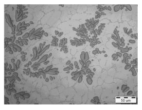
Fig. 6. Microstructure of *CuNb15* alloy ingot, section perpendicular to casting direction.
