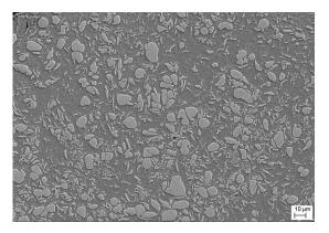
Fig. 14. Microstructure of *CuNb15* alloy wire after drawing to diameter of 0.5 mm and after annealing in temperature of 700 °C for 3 hours, section perpendicular to drawing direction.
