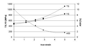
Fig. 3. Changes in mechanical properties (TS-tensile strength, YS-yield strength, A50-elongation ) of *CuAg15* wire vs. true strain
