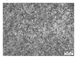
Fig. 1. Microstructure of CuAg15 ingot.
