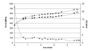
Fig. 8 Changes in mechanical properties (TS-tensile strength, YS-yield strength, A100-elongation) of *CuNb15* wire vs. true strain of cold deformation
