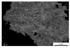
Fig. 21. Nanostructure of niobium filament in *CuNb15k* composite after drawing down to diameter of 0.15 mm. True strain  $\varepsilon = 5.83$
