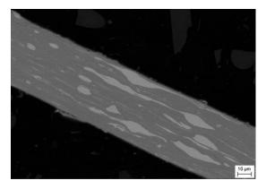
Fig. 11. Microstructure of *CuNb15* alloy wire after drawing to diameter of 0.087 mm, section parallel to drawing direction
