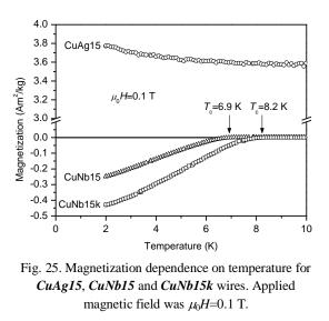
Better composition of CuNb15k composite wire and absence of inclusions or pollutions of the normal phases inside the Nb filaments results in higher critical temperature which is about  $T_c=8.2$  K and approaches the critical temperature of pure Nb (9.2 K).
