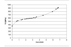
Fig. 9. Changes in tensile strength of *CuNb15* wire vs. true strain of cold deformation
