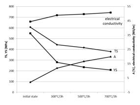
Fig. 15. Changes of tensile strength (TS) yield strength (YS) elongation (A) and electrical conductivity of *CuNb15* alloy wire of diameter 0.5 mm vs. annealing temperature.
