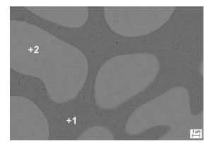
Fig. 7. Microstructure *CuNb15* alloy ingot with content of alloying elements in microsections (EDS): +1 Cu = 100%, +2 Nb = 96.2%; Cu = 3.8%
