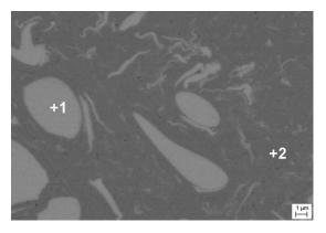
Fig. 12. Microstructure of *CuNb15* alloy wire after drawing to diameter of 0.087 mm with content of alloying elements in microsections (EDS), section perpendicular to drawing direction +1 Nb = 93.98%; Cu = 6.02%, +2 Nb = 5.95%; Cu = 94.05%.
