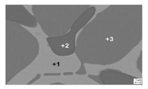
Fig. 2. Microstructure of *CuAg15* ingot with chemical composition analysis (EDS) in microsections (polished section):
