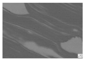
Fig. 10. Microstructure of *CuNb15* alloy wire after drawing to diameter of 0.5 mm, section parallel to drawing direction
