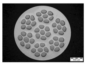
Fig. 17. Section of *CuNb15k* composite after third compacting stage
