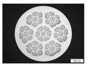
Fig. 18. Section of *CuNb15k* composite after fifth compacting stage
