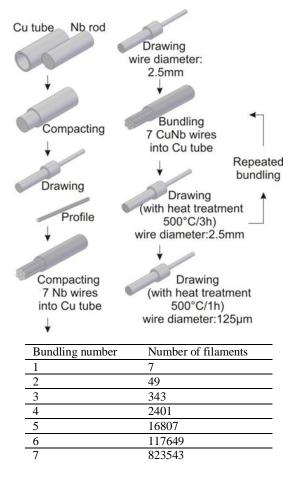
Fig. 16. Production of *CuNb15k* composite with defined number of filaments in individual stages of compacting.
