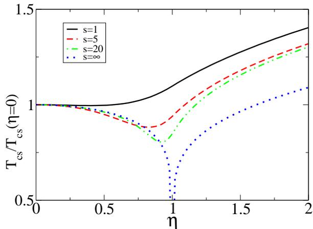
FIG. 6: Variation of the scaled critical temperature of spin  $s$  bosons  $T_{cs}/T_{cs}(\eta=0)$  with increasing  $\eta$ , for fixed parameter  $\chi = 3$ . Different lines represent different spin  $s$  of the bosons. Analytical result of the critical temperature  $T_{\infty}/T_{\infty}(\eta=0)$  in the limit of  $s \rightarrow \infty$  using the Dicke model (Eq. 42) is shown by the dotted line.
