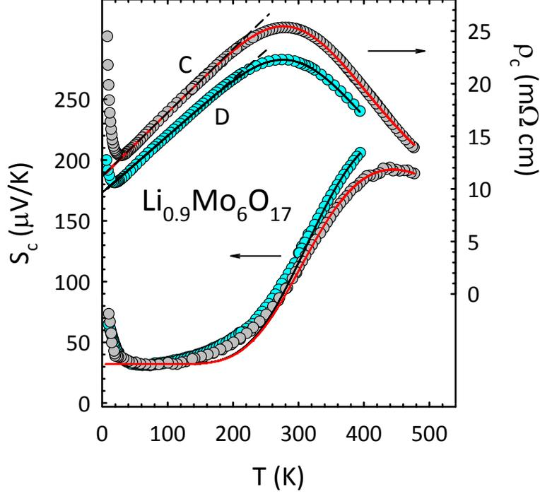
FIG. S1. LiPB inter-chain ( $c$ -axis) thermopowers (left ordinate) and resistivities (right ordinate) for crystals C and D. Solid curves through the data are fits to the parallel conduction model discussed in the text; parameters for the semiconducting component are listed in Table I. Dashed lines are linear-least-squares fits to the low- $T$   $\rho_c(T)$ .
