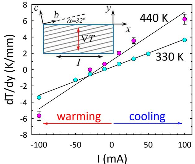
FIG. 3. (color online) Current dependence of the transverse Peltier-induced temperature gradient for a LiPB crystal at  $T = 330$  K and 440 K. Error bars reflect uncertainty due to slow oscillations in the Cu block temperature ( $\leq 0.1$  K), particularly at the highest  $T$ . The inset shows the orientation of current and heat flow relative to the specimen ( $x$ - $y$ ) and crystallographic ( $b$ - $c$ ) axes.
