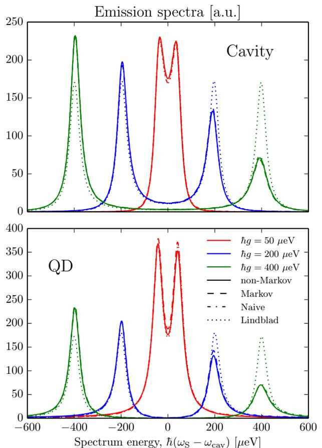
FIG. 17. Emission spectra, Eq. (39), comparing the NM2PT with various approximations. Parameters:  $\hbar\Delta = 0$ ,  $\hbar\Gamma = 1 \mu\text{eV}$ ,  $\hbar\kappa = 100 \mu\text{eV}$ ,  $\hbar\gamma = 0$ ,  $l_g = l_e = 5 \text{ nm}$ , and  $T = 4 \text{ K}$ .
