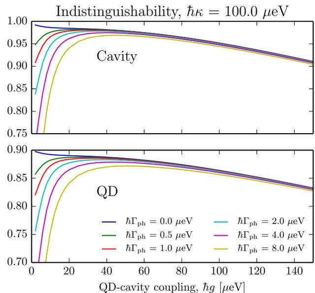
FIG. 11. Dependence of cavity (top) and QD (bottom) indistinguishability on phonon lifetime as a function of QD-cavity coupling. Parameters:  $\hbar\kappa = 100$   $\mu\text{eV}$ ,  $\hbar\Delta = 0$ ,  $\hbar\Gamma = 1$   $\mu\text{eV}$ ,  $\hbar\gamma = 0$ ,  $l_g = l_e = 5$  nm, and  $T = 4$  K. See Fig. 12 for more  $\kappa$  values
