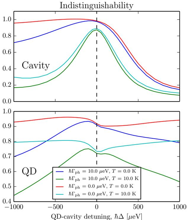
FIG. 15. Dependence of cavity (top) and QD (bottom) indistinguishability on QD-cavity detuning  $\Delta$ . Parameters:  $\hbar\kappa = 100 \mu\text{eV}$ ,  $\hbar g = 100 \mu\text{eV}$ ,  $\hbar\Gamma = 1 \mu\text{eV}$ , and  $l_h = l_e = 5 \text{ nm}$ .
