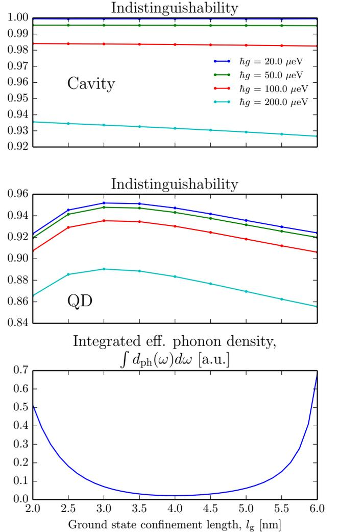
FIG. 14. Dependence of cavity (top) and QD (middle) indistinguishability on confinement lengths. The excited state confinement length is chosen so that  $l_e^3 + l_g^3 = 2 \times (5 \text{ nm})^3$  is fixed. Frequency integral (bottom) over the effective phonon density, Eq. (19),  $\int d_{\text{ph}}(\omega) d\omega$ . Parameters:  $\hbar\kappa = 100 \mu\text{eV}$ ,  $\hbar\Delta = 0$ ,  $\hbar\Gamma = 1 \mu\text{eV}$ ,  $\hbar\gamma = 0$ , and  $T = 4$  K.
