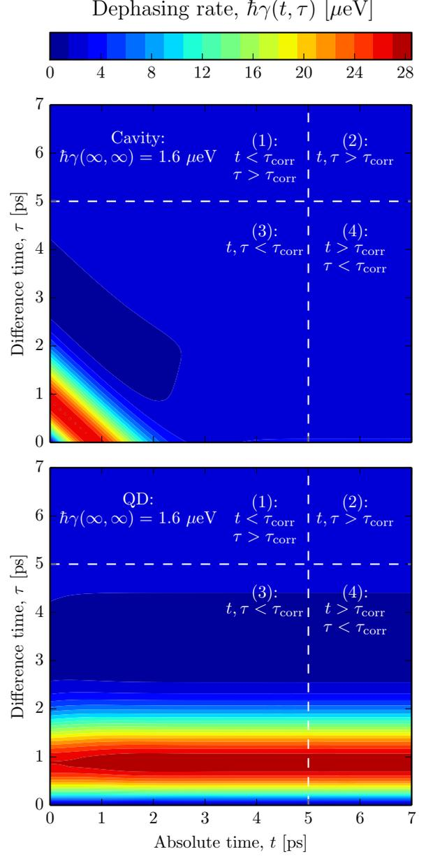
FIG. 7. Real part of time-dependent two-time dephasing rates for QD, Eq. (29), and cavity, Eq. (28). Parameters:  $\hbar g = 100 \mu\text{eV}$ ,  $\hbar\Delta = 0$ ,  $T = 4$  K, and  $l_h = l_e = 5$  nm.
