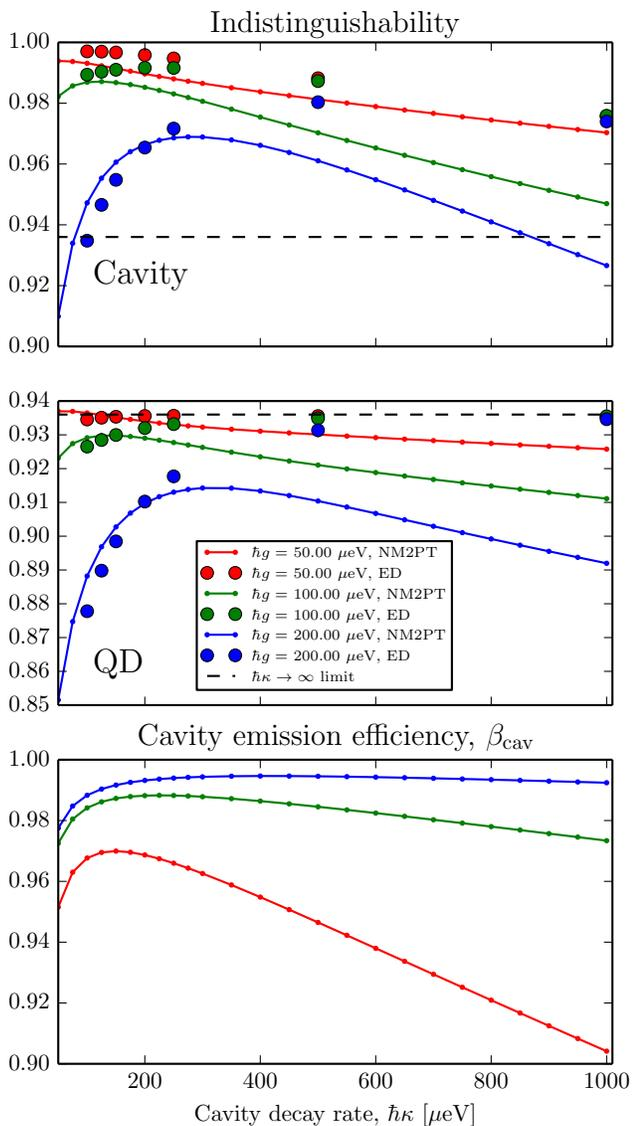
FIG. 4. Indistinguishability (two upper plots) as a function of the cavity decay rate, calculated from Eq. (7) and using an exact diagonalization (ED) approach<sup>22,28,29</sup> and cavity emission efficiency  $\beta_{\text{cav}}$ , see Eq. (22) (lower plot). Parameters:  $\hbar\Gamma = 1 \mu\text{eV}$ ,  $\hbar\Delta = 0$ ,  $T = 0 \text{ K}$ , and  $l_h = l_e = 5 \text{ nm}$ .
