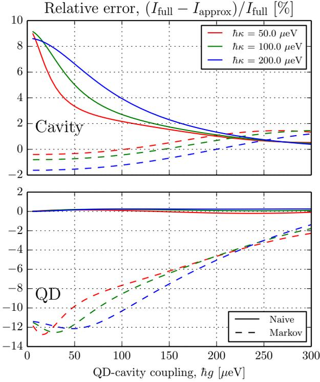
FIG. 16. Relative error of the indistinguishability for various approximations, see main text. Parameters:  $\hbar\Gamma = 1 \mu\text{eV}$ ,  $T = 4 \text{ K}$ ,  $\hbar\Delta = 0$ , and  $l_h = l_e = 5 \text{ nm}$ .
