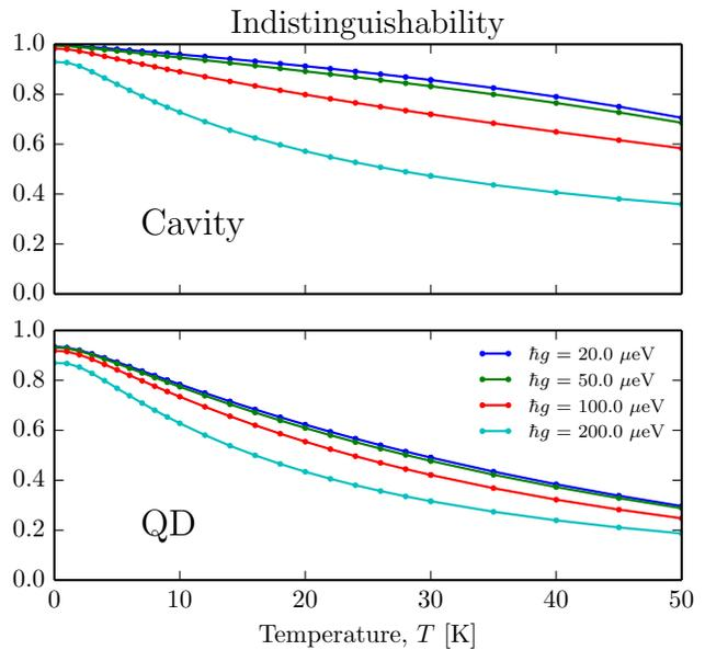
FIG. 9. Temperature dependence of cavity (top) and QD (bottom) indistinguishability. Parameters:  $\hbar\kappa = 100 \mu\text{eV}$ ,  $\hbar\Delta = 0$ ,  $\hbar\Gamma = 1 \mu\text{eV}$ ,  $\hbar\gamma = 0$ ,  $l_g = l_e = 5 \text{ nm}$ .
