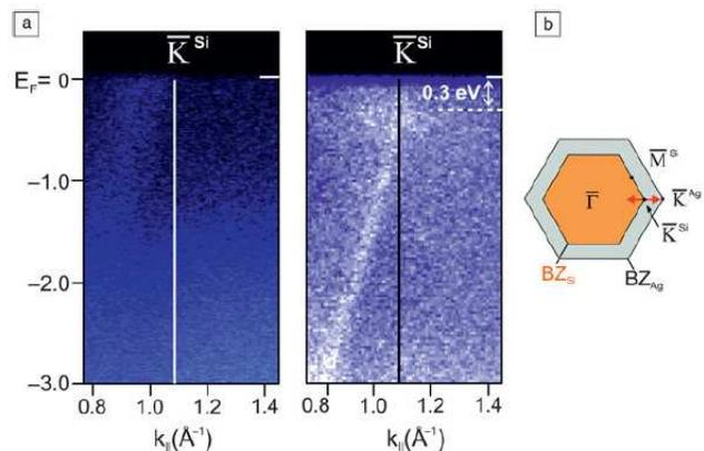
FIG. 5. (a) Angle-resolved photoelectron spectroscopy of a clean silver surface (left) and with silicene coverage (right); (b) Brillouin zone showing the location of various points. Reprinted with permission from Reference [11]. ©2012 American Physical Society.
