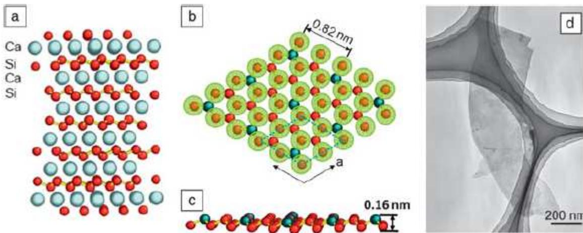
FIG. 1. (a) Model of  $\text{CaSi}_2$ ; (b-c) top and side view of Mg-doped silicon sheet capped with oxygen; (d) TEM image of nanosheet. Reprinted with permission from Reference [5]. ©2006 Wiley-VCH Verlag GmbH & Co. KGaA, Weinheim.
