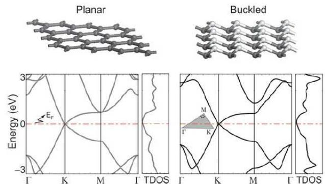
FIG. 4. Band structure of flat and buckled silicene. Reprinted with permission from Reference [19]. ©2005 American Physical Society. TDOS, total density of states.
