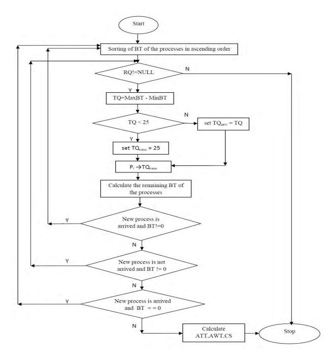
Figure 2. Flowchart of Min-Max Round Robin (MMRR) algorithm
