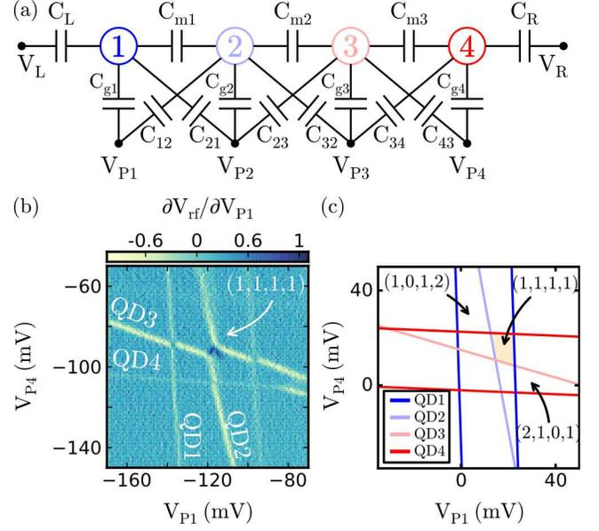
FIG. 2. (Color online) (a) Schematic of the QD capacitive model used throughout this paper to calculate the charge stability diagrams. (b) Charge stability diagram close-up of the  $(1,1,1,1)$  region, in the plane defined by plunger gates  $P_1$  and  $P_4$ , with  $V_{P_2} = -40$  mV and  $V_{P_3} = -180$  mV. (c) Calculated transition lines using the model of (a) and  $C_{gi} = C_{mi} = C_L = C_R = 10$  aF and  $C_{i\pm 1,i} = 1$  aF for  $i = 1, 2, 3, 4$ .
