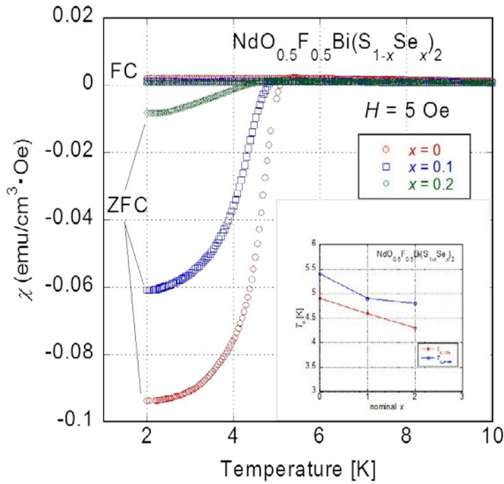
Fig. 3 Temperature dependences of the magnetic susceptibility ( $\chi$ ) of  $\text{NdO}_{0.5}\text{F}_{0.5}\text{Bi}(\text{S}_{1-x}\text{Se}_x)_2$  ( $x = 0, 0.1, 0.2$ ).
