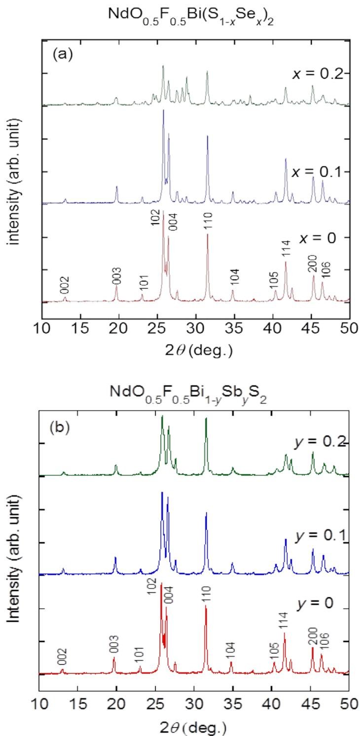
Fig. 1 XRD patterns of (a)  $\text{NdO}_{0.5}\text{F}_{0.5}\text{Bi}(\text{S}_{1-x}\text{Se}_x)_2$  ( $x = 0, 0.1, 0.2$ ) and (b)  $\text{NdO}_{0.5}\text{F}_{0.5}\text{Bi}_{1-y}\text{Sb}_y\text{S}_2$  ( $y = 0, 0.1, 0.2$ ).
