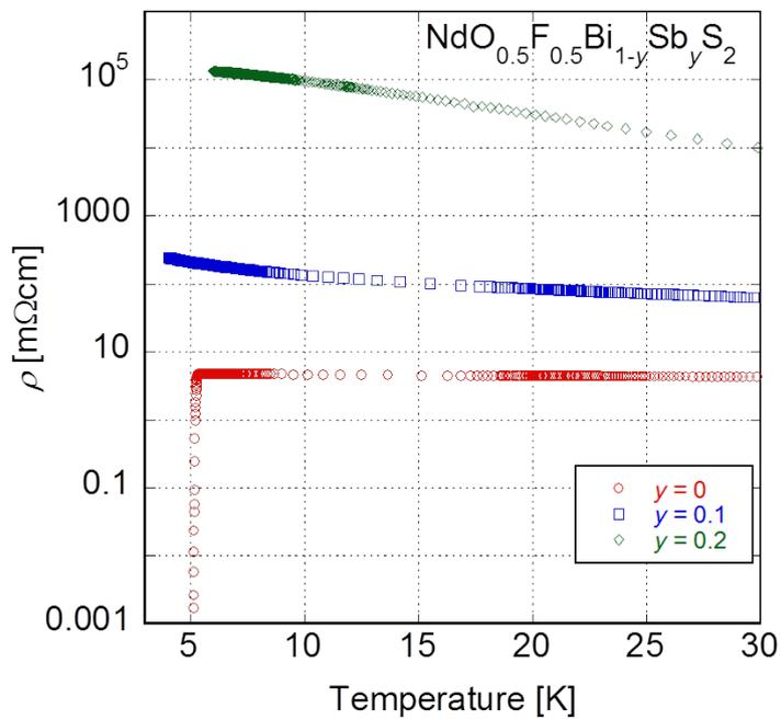
Fig. 4 Temperature dependences of electrical resistivity ( $\rho$ ) of  $\text{NdO}_{0.5}\text{F}_{0.5}\text{Bi}_{1-y}\text{Sb}_y\text{S}_2$  ( $y = 0, 0.1, 0.2$ ).
