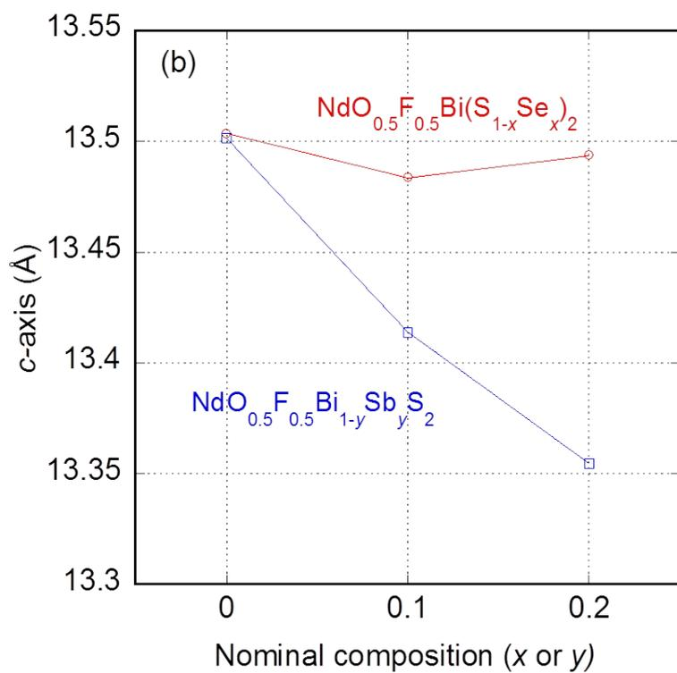
Fig. 2 Se-concentration  $x$  dependence (or Sb-concentration  $y$  dependence) of the lattice constants of (a)  $a$ -axis and (b)  $c$ -axis.
