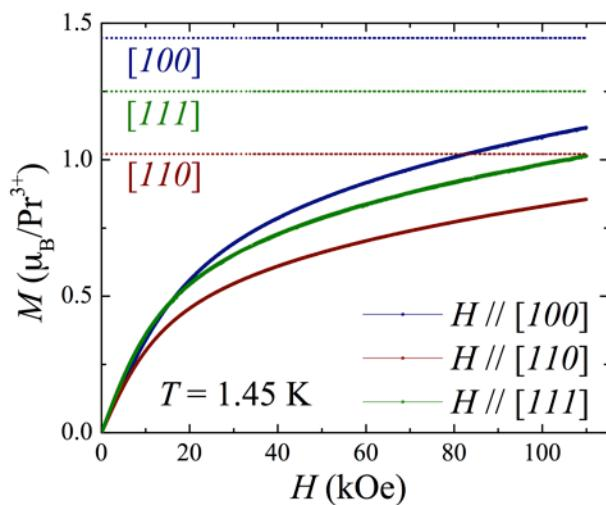
Figure 6. Isothermal magnetization ( $M$ ) at  $T = 1.45$  K of a crystal of  $\text{Pr}_2\text{Zr}_2\text{O}_7$ , along the [100], [110], and [111] directions, plotted as a function of applied magnetic field ( $H$ ).
