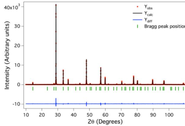
Figure 1. Room temperature powder X-ray diffraction pattern (in red) of the stoichiometric polycrystalline rod of  $\text{Pr}_2\text{Zr}_2\text{O}_7$  used for the crystal growth. Also shown are the fit to the cubic  $F\bar{d}3m$  structure (in black) and the difference curve (in blue).
