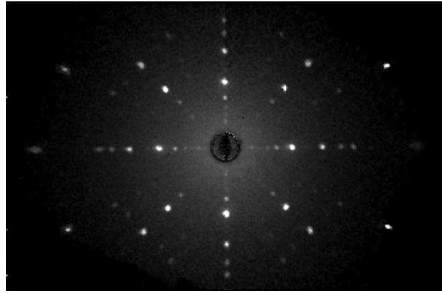
Figure 3. X-ray Laue back reflection photograph of a crystal of  $\text{Pr}_2\text{Zr}_2\text{O}_7$ , grown from a starting composition with no  $\text{Pr}_6\text{O}_{11}$  excess, showing the [100] orientation.
