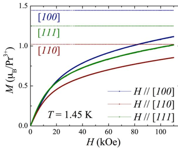
Figure 6. Isothermal magnetization ( $M$ ) at  $T = 1.45$  K of a crystal of Pr<sub>2</sub>Zr<sub>2</sub>O<sub>7</sub>, along the [100], [110], and [111] directions, plotted as a function of applied magnetic field ( $H$ ).
