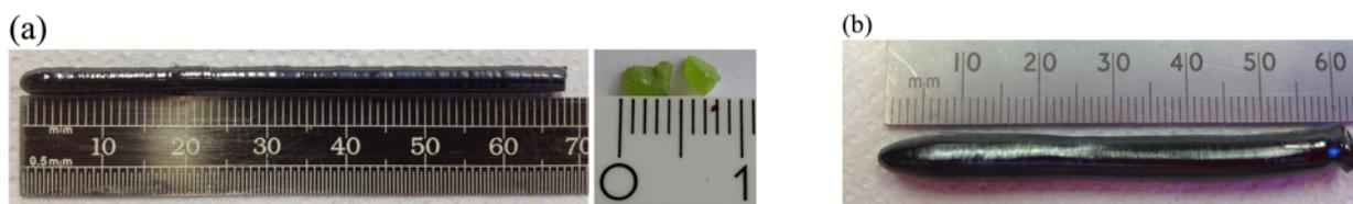
Figure 2. Single crystals of  $\text{Pr}_2\text{Zr}_2\text{O}_7$  grown by the floating zone method, (a) part of a boule grown from a stoichiometric starting composition (with no  $\text{Pr}_6\text{O}_{11}$  excess), in 1 bar oxygen pressure at 15 mm/h. Inset: a few pieces from the boule annealed in Ar +3%  $\text{H}_2$  flow for 2 days, (b) boule grown from a starting composition with a 10%  $\text{Pr}_6\text{O}_{11}$  excess in 4 bar oxygen pressure at 15 mm/h.
