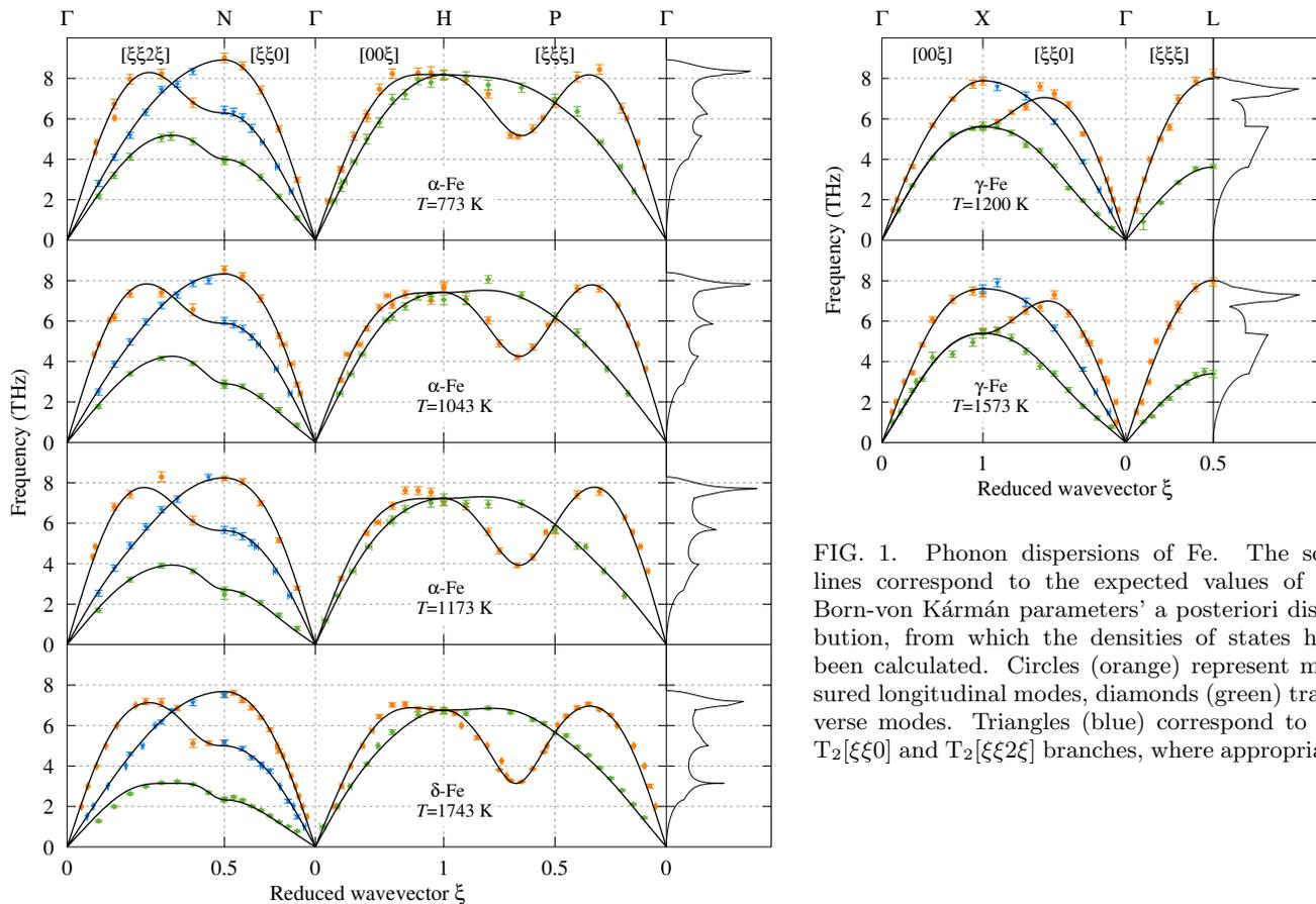
FIG. 1. Phonon dispersions of Fe. The solid lines correspond to the expected values of the Born-von Kármán parameters' a posteriori distribution, from which the densities of states have been calculated. Circles (orange) represent measured longitudinal modes, diamonds (green) transverse modes. Triangles (blue) correspond to the  $T_2[\xi\xi 0]$  and  $T_2[\xi\xi 2\xi]$  branches, where appropriate.
