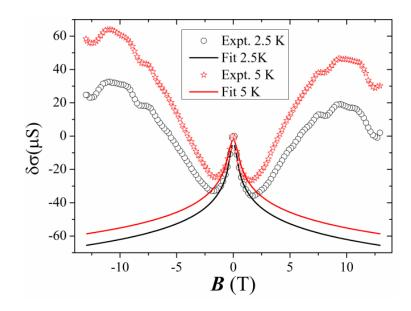
**Fig. 3** The magnetoconductance at 2.5 K and 5 K, which in low field, can be fitted by the HKN formula.
