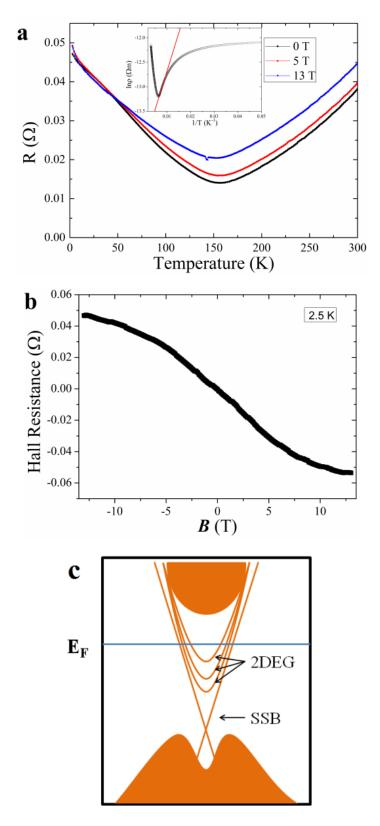
**Fig. 1** (a) Temperature dependence of the resistance at 0, 5, and 13 T. Below around 150 K, the resistance shows insulating temperature dependence. The inset contains the corresponding Arrhenius plot. (b) Hall resistance of the single crystal measured at 2.5 K. (c) Schematic diagram of the band structure for  $BiSbTe_3$  single crystal. The Fermi level is located in the bulk band gap but close to the conduction band, and the 2DEG subbands are inferred from the crossover from WAL to WL.
