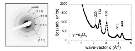
*Figure S1*: Microdiffraction spectrum obtained for iron oxide nanoparticles (left). Wave-vector dependence of the scattering intensity obtained for iron oxide nanoparticles (right).
