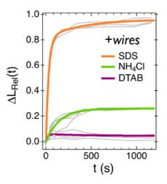
**Figure S6**: Relative length increase  $\Delta L_{Rel}(t)$  of positive wires submitted to solutions containing anionic (SDS, 0.96 wt. %), to cationic (DTAB, 10 wt.%) and to 2 M NH<sub>4</sub>Cl solutions. Data in grey are those of individual objects, and the colored lines represent the average.
