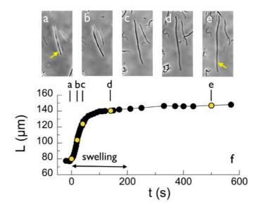
**Figure 2:** Swelling kinetics of positively charged wires exposed to a sodium dodecyl sulfate solution at a concentration of 0.96 wt. % and a flow rate of 100  $\mu$ L/min. a-e) Snapshots of wires at t = 0, 20, 40, 140 and 500 s, respectively. f) Relative length increase  $\Delta L_{Rel}(t)$  of the wire shown by an arrow in a) and e). The length goes from 80  $\mu$ m to 150  $\mu$ m in the stationary state, corresponding to  $\Delta L_{Rel} = 0.94$ .
