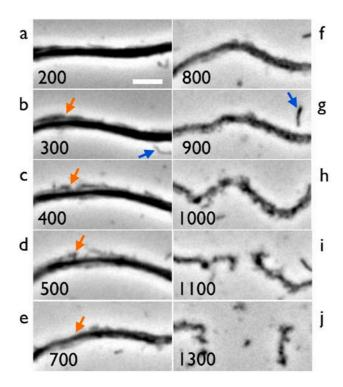
**Figure 5**: Close-up views of a wire during disassembly. The bar in the first image is 3  $\mu$ m. Note that as time evolves the outer surface becomes irregular, the diameter increases and large pieces detach from the structure. Detached aggregates indicated by arrows are about one micron in size.
