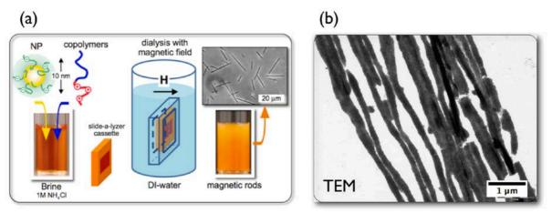
*Figure S3: a)* Schematic representation of the protocol that controls the nanoparticle co-assembly and wire formation. b) image of wires aggregated on a TEM grid.
