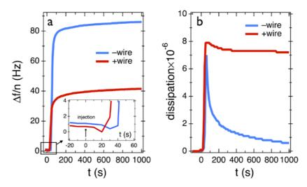
**Figure 6**: a) Frequency shift  $\Delta f(t)$  for both negative and positive wires when exposed to a 0.48 wt. % SDS solution. The increase of the frequency shift after the injection of SDS is interpreted as a loss of materials from the surface. Inset: close-up view of the initial frequency shift showing a small but measurable negative undershoot. b) Time evolution of the dissipation  $\Delta D$  associated with the behavior of Fig. 6a.
