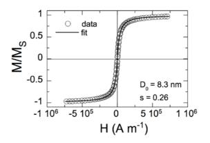
**Figure S2:** Magnetic field dependence of the macroscopic magnetization M(H) normalized by its saturation value  $M_s$  for cationic maghemite dispersions. The solid curve was obtained using the Langevin function for superparamagnetism convoluted with a log-normal distribution function for the particle sizes, given with median
