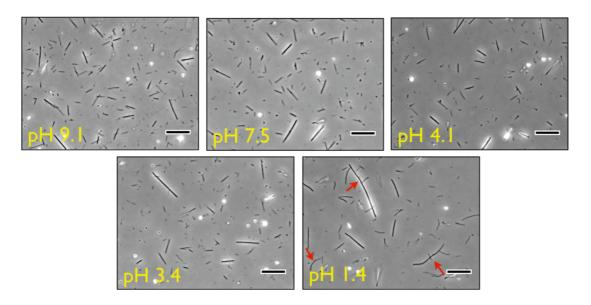
Figure S5 : Phase-contrast images of magnetic nanowires at different pH.
