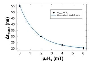
FIG. 3. Graph showing the minimum length of the current pulse needed in order to switch the magnetization in at least 10 of the 20 nanowires of the sample, as function of the longitudinal magnetic field. The pulse current density is  $5.8 \times 10^{11}$  A/m<sup>2</sup>. We observe successful magnetization switching at zero field, for current pulses of at least 55 ns in length. The fitting curve is based on the generalized Néel-Brown model for thermal-assisted magnetization switching.
