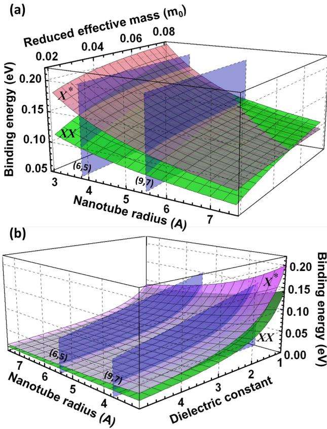
FIG. 3: (Color online) Trion ( $X^*$ ) and biexciton ( $XX$ ) binding energies given by Eqs. (8) and (2) with  $|E_X| = Ry^*/r^{0.6}$ , as functions of the CN radius and  $\mu$  with  $\varepsilon = 1$  (a), and as functions of the CN radius and  $\varepsilon$  with  $\mu = 0.04$  (b). Vertical parallel planes indicate the radii of the (6,5) and (9,7) CNs studied experimentally.
