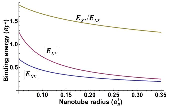
FIG. 2: (Color online) Trion binding energy, biexciton binding energy and their ratio given by Eqs. (8), (2) and (9), respectively, with  $|E_X| = Ry^*/r^{0.6}$  (Ref. [22]) as functions of the dimensionless nanotube radius.
