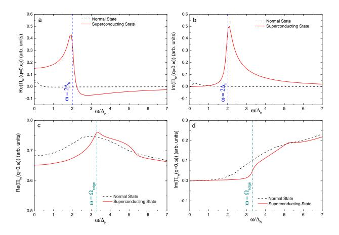
FIG. 6: (Color online) Real and Imaginary parts of polarizability  $\Pi(\mathbf{q} = \mathbf{0}, \omega)$  in Normal and Superconducting state. (a-b) Standard intraband polarizability  $\Pi_{(hh)}$ . (c-d) Interband polarizability  $\Pi_{(he)}$ .
