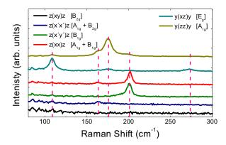
FIG. 1: Room temperature Raman spectra on NaFeAs in z(xy)z, z(x'y')z, z(x'x')z, z(xx)z, y(xz)y, and y(zz)y configurations. Spectra have been shifted vertically for clarity. Starting from the left, the peaks are assigned to the  $E_g(As)$ ,  $A_{1g}(As)$ ,  $A_{1g}(Na)$ ,  $B_{1g}(Fe)$  and  $E_g(Fe)$  modes.
