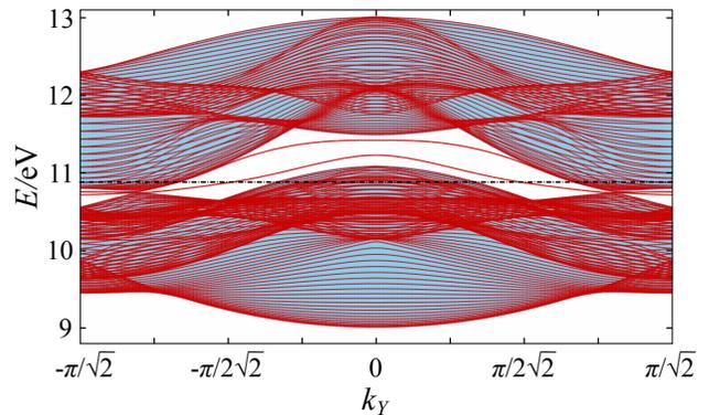
FIG. 8. (Color online) Energy bands in the paramagnetic phase for the five-orbital model. Bands of a (11) strip of width  $W = 20$  (red) are compared to the bulk bands projected onto the 1D BZ for the strip (blue). The black dash-dotted line denotes the Fermi energy at filling factor 0.6.
