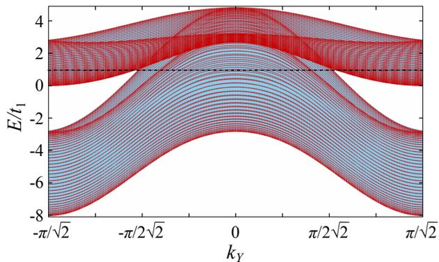
FIG. 6. (Color online) Energy bands in the paramagnetic phase for the two-orbital model. Bands of a (11) strip of width  $W = 40$  (red) are compared to the bulk bands projected onto the 1D BZ for the strip (blue). The black dash-dotted line denotes the Fermi energy at half filling.
