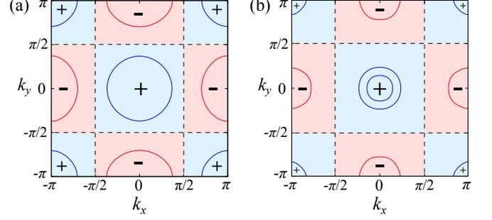
FIG. 1. (Color online) Sign structure of the superconducting gap function with  $s_{\pm}$ -wave structure. The red (blue) areas denote regions in the BZ where the sign of  $\cos k_x \cos k_y$  is negative (positive). The dashed lines show the nodes of this function. In addition, the Fermi surfaces of (a) the two-orbital model and (b) the five-orbital model are plotted.
