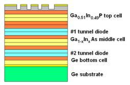
Figure 1 GaInP/GaAs/Ge photovoltaic cell structure
