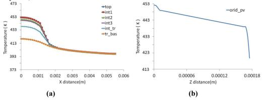
Figure 10 Temperature profile at 170s mapped onto paths (a) along X and (b) Z axis
