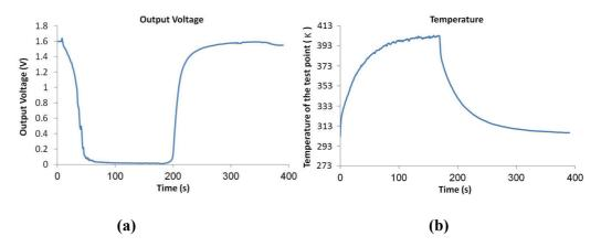
Figure 3 (a) Output voltage fluctuation and (b) temperature history of the photovoltaic cell
