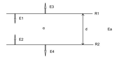
Figure 4 Light reflection, transmission and absorption in any monolayer
