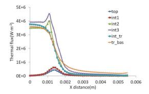
Figure 11 Thermal flux profile at 170s mapped onto path along X axis
