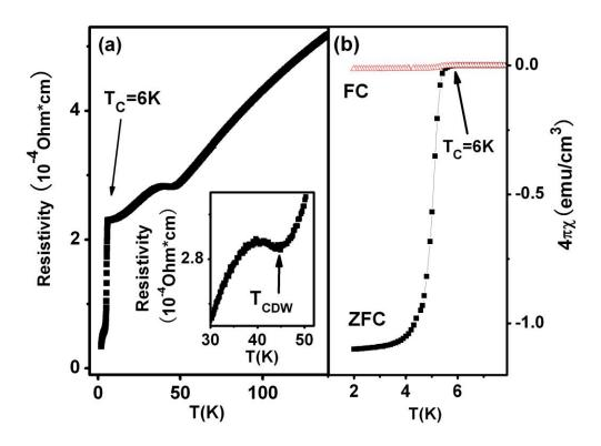
Fig. 2 (a) Temperature dependence of resistivity for the as-prepared  $BaTi_2(Sb_{0.84}Bi_{0.16})_2O$ . The expanded plot shown in the inset indicates the CDW/SDW anomaly below about 44K. (b) Temperature dependence of ZFC (solid squares) and FC (hollow triangles) magnetic susceptibilities of as-prepared  $BaTi_2(Sb_{0.84}Bi_{0.16})_2O$ .
