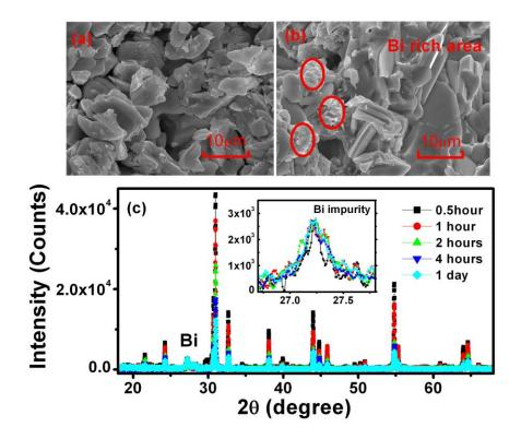
**Fig. 1** SEM images of BaTi<sub>2</sub>(Sb<sub>0.84</sub>Bi<sub>0.16</sub>)<sub>2</sub>O exposed to air for about one hour, with (a) representing to the most extent the typical texture features without Bi impurity and (b) the area where little Bi impurity can be detected in very limited local grain boundary, as indicated by the circles. (c) Powder X-ray diffraction patterns for samples with various exposure durations.
