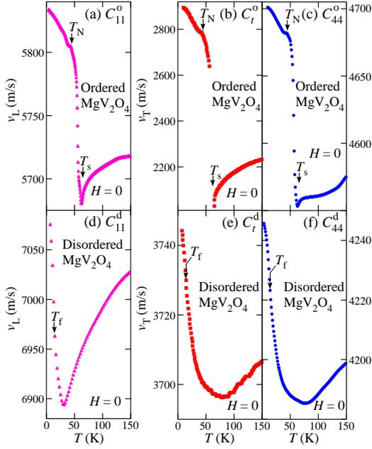
FIG. 1: (Color online).  $T$  dependence of  $v_L$  and  $v_T$  with  $H = 0$  in  $\text{MgV}_2\text{O}_4$ . (a)-(c) The ordered  $\text{MgV}_2\text{O}_4$ : (a)  $C_{11}^o$ , (b)  $\frac{(C_{11}^o - C_{12}^o)}{2} \equiv C_t^o$ , and (c)  $C_{44}^o$ .  $T_s$  and  $T_N$  are marked by arrows in (a)-(c). (d)-(f) The disordered  $\text{MgV}_2\text{O}_4$ : (d)  $C_{11}^d$ , (e)  $C_t^d$ , and (f)  $C_{44}^d$ .  $T_f$  is marked by arrows in (d)-(f).
