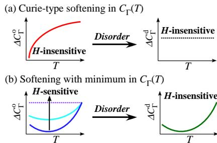
FIG. 3: (Color online). Schematic of the two-types of the elastic anomalies in the cubic PM phase of  $\text{MgV}_2\text{O}_4$ . (a) Disorder-sensitive Curie-type softening in  $C_T(T)$  and (b)  $H$ - and disorder-sensitive softening with minimum in  $C_T(T)$ .
