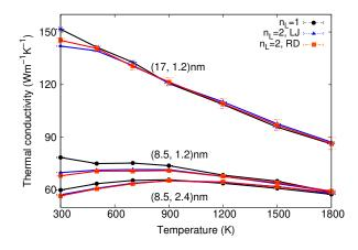
FIG. 5: (Color online) The thermal conductivity versuses temperature in single-layer graphene and bilayer graphene of various dimensions. The LJ and RD potentials result in a close value of thermal conductivity in bilayer graphene.
