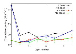
FIG. 7: (Color online) The thermal conductivity v.s the number of layers in FLG of dimension  $8.5 \times 1.2$  nm. The LJ and RD potentials give close value of thermal conductivity for all FLG. Note the distinct reduction in the thermal conductivity for number increasing from 1 to 2 at 300 K. At high temperature (1200K), the thermal conductivity becomes insensitive to the layer number.
