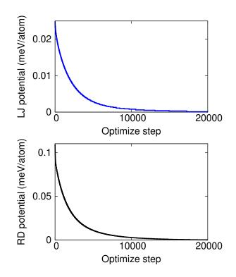
FIG. 2: (Color online) The decrease of the total LJ potential or the RD potential during the structure relaxation in bilayer graphene of dimension  $8.5 \times 1.2$  nm. The structure is relaxed by the simple steepest method. The initial configuration is an AB-stacking bilayer graphene with interlayer space 0.335 nm and intralayer bond length 0.142 nm.
