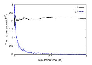
FIG. 4: (Color online) Thermal current across the bilayer graphene of dimension  $8.5 \times 1.2$  nm at room temperature.
