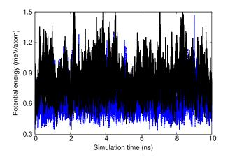
FIG. 6: (Color online) The LJ (blue online) and RD (black online) potential energies during MD simulation in bilayer graphene of dimension  $8.5 \times 1.2$  nm. The energy is with reference to the value at equilibrium configuration. The RD potential energy is higher than the LJ potential, but they are on the same order.
