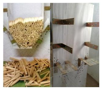
Figure 1.1 Two-dimensional model silo. Front view (left), silo filled with wood particles and a hopper configuration; and side view (right), silo empty of particles and a flat-bottom silo configuration.
