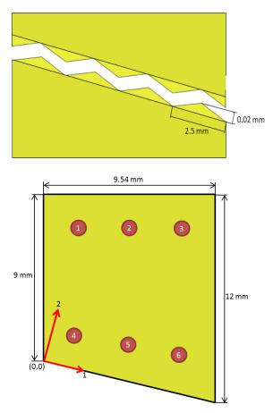
Figure 3.5 (top) Model for rough surface used in the finite element calculation; (bottom) markers used to calculate stress and displacements as listed in Table 3.1.
