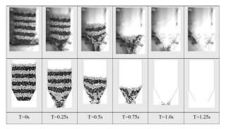
Figure 4.5 Snapshots in the experiments (top) and simulation (bottom) in the A4 silo.
