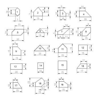
Figure 4.2 Cross-sectional shapes of wood particles (dimensions in mm
