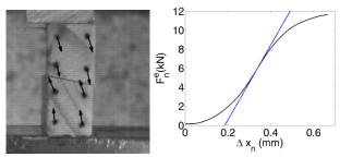
Figure 3.2 (left) Miniature triaxial test used to measure load-displacement relation; (right) between two wood particles.
