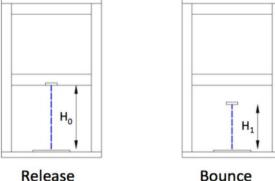
Figure 3.7 Apparatus used to determine the particlewall coefficient of restitution.
