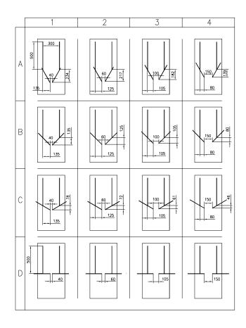
Figure 4.1 Geometrical configurations of the model silo (dimensions in mm).
