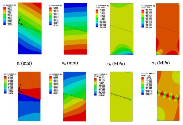
Figure 3.6 Top images are for flat surfaces with friction coefficient of 0.37; bottom images are for rough surfaces with friction coefficient of 0.2. Pairs from left to right: tangential displacement, normal displacement, tangential stress, and normal stress.
