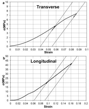
Figure 3.3 Stress versus strain in loading-unloading cycles in (top) transverse direction and (bottom) longitudinal direction, relative to wood fibres.
