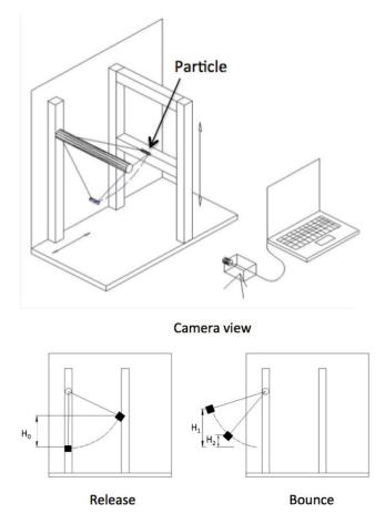
Figure 3.8 Apparatus used to determine the particleto-particle coefficient of restitution.
