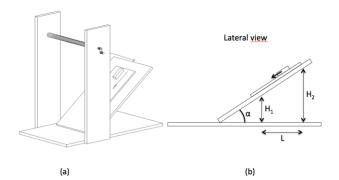
Figure 3.1 Apparatus used to determine the particleto-wall and particle-to-particle coefficients of friction; general view (a) and detailed view (b).
