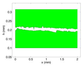
Figure 3.4 Topography of particle surfaces: top line shows transverse direction (perpendicular to fibres); and bottom line, longitudinal (parallel to fibres).
