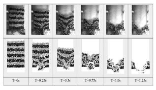
Figure 4.6 Snapshots in the experiments (top) and simulation (bottom) in the D4 silo.
