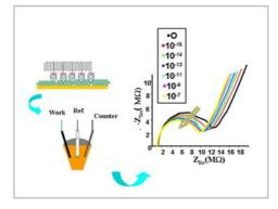
Figure 1. Schematic representation of EIS measurements performed on samples of rat OR -I7 at increasing concentrations of the specific odorant, octanal. On the left: the sample and the electrochemical cell; on the right: the experimental results. The straight arrow indicates the increasing concentration of octanal.
