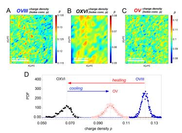
**Figure 4.** (colored on-line): **(a)**, **(b)** and **(c)** The spatial map of the charge density (holes concentration p) of the OVIII, OXVI and OV puddles, have been reported. **(d)** Distribution of the charge density into the OVIII (blue filled circles), OXVI (black filled squares) and OV (red empty crosses) puddles. During the thermal annealing process the charge density changed and its distribution in the OXVI and OV puddles get broader.
