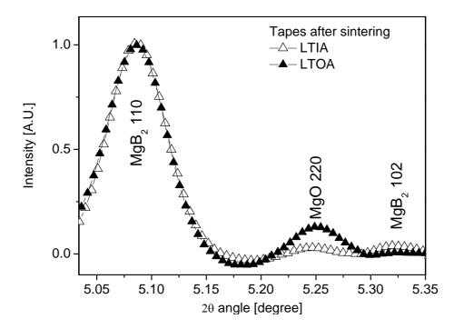
**Figure 8.** Enlarged view of the HEXRD patterns of samples synthesised under different atmosphere (IA and OA) both at low temperature (LT), the patterns have been acquired during the sintering process of respective tapes, here only the last pattern for each is reported.
