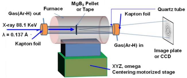
Figure 1. Experimental set-up for the transmission HEXRD analysis at ID11 beamline of ESRF.
