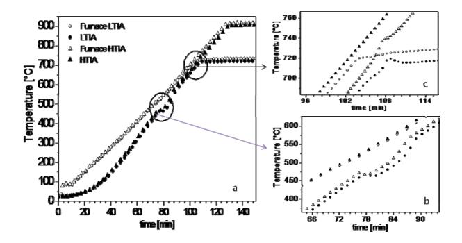
**Figure 2.** Thermal analysis of the  $MgB_2$  synthesis reaction (a) temperature profile of the thermal treatments for the low and high synthesis temperature. (b) details of  $MgH_2$  decomposition and of  $MgB_2$  formation (c).
