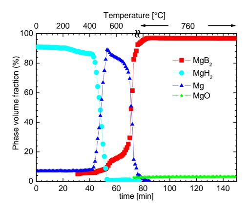
Figure 3. Phase volume fraction evolution as a function of the time during the synthesis of MgB<sub>2</sub> at low temperature  $(760^{\circ}C)$ .
