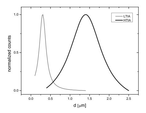
**Figure 4.** granulometry distribution fitted with a Lorentzian function for the low temperature synthesis sample (LTIA) and for the high temperature synthesis (HTIA) one.
