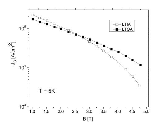
Figure 9. Magnetic  $J_c$  of the sample synthesized at low temperature in different atmosphere reference [7].
