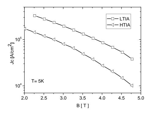
**Figure7.**  $J_c$  measurements for the wires of reference [5] (synthesis temperature for LTIA = 745°C).
