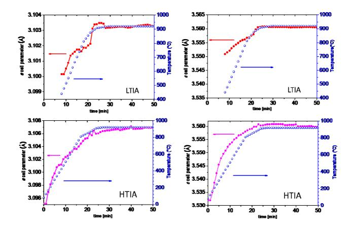
Figure 5.  $MgB_2$  lattice parameters evolution during the sintering process for LTIA (upper panel) and HTIA (lower panel) samples.
