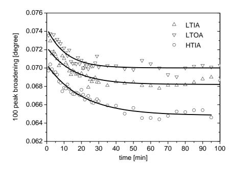
Figure 6. Broadening of the 100 peak of  $MgB_2$  as a function of sintering time for different synthesis temperature and atmosphere. The continuous lines represent the exponential fit of each data set.
