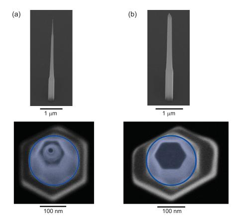
FIG. 4. Nanowire birefringence. SEM images of: (a) symmetric nanowire waveguide, and (b) asymmetric nanowire waveguide. Top panel: side-view SEM images of nanowires with tilt angle of 45 degrees. Bottom panel: SEM images of the nanowires viewed from the top at a small tilt angle. The blue shaded circle represents the opening in the SiO2 mask. The example of the nanowire elongation in (b) is an extreme example that leads to geometric birefringence and corresponding rotation of the quantum state.
