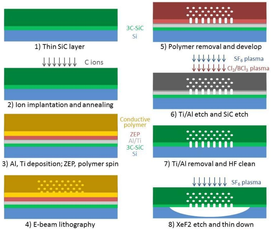
Fig 2: Photonic crystal fabrication process starting from a 300 nm thick 3C silicon carbide epilayer on a 100 mm silicon wafer.
